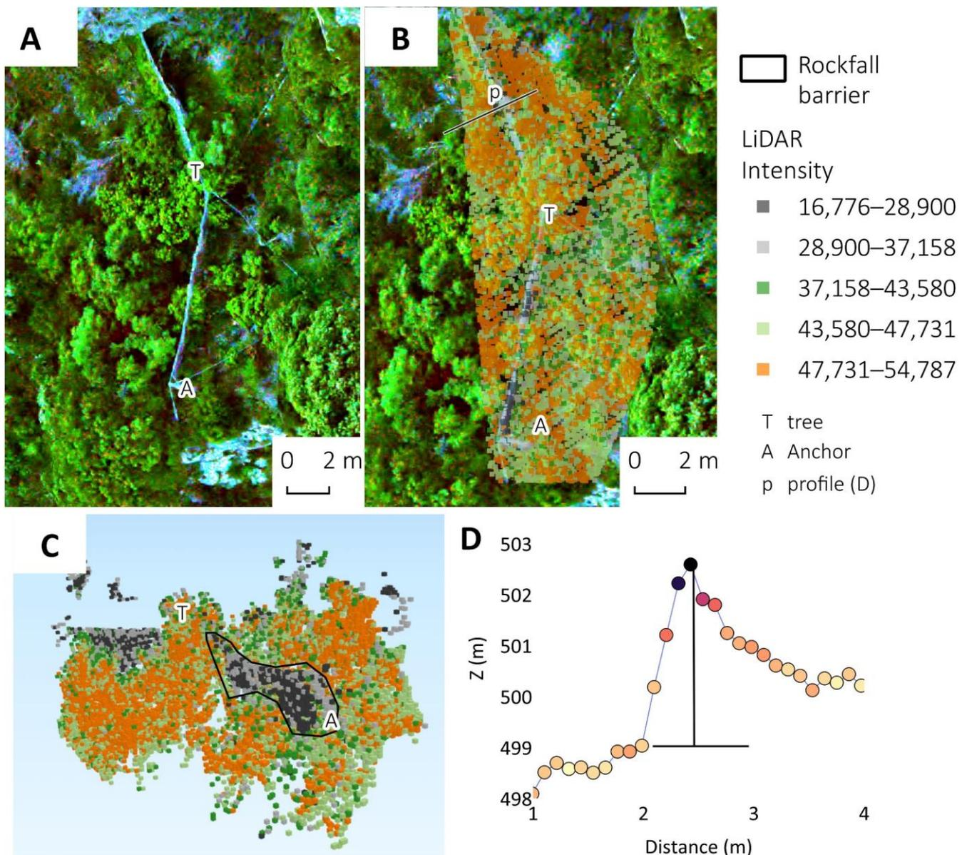
**Figure 7.** An example of a rockfall barrier in a steep slope detected on orthophoto and confirmed by LiDAR point cloud. (A) Orthophoto with 10 cm of spatial resolution. (B) Sampled LiDAR point cloud classified by intensity. (C) A 3-D view of the LiDAR point cloud. (D) Vertical barrier profile based on LiDAR data interpolated in 10 cm DSM.
