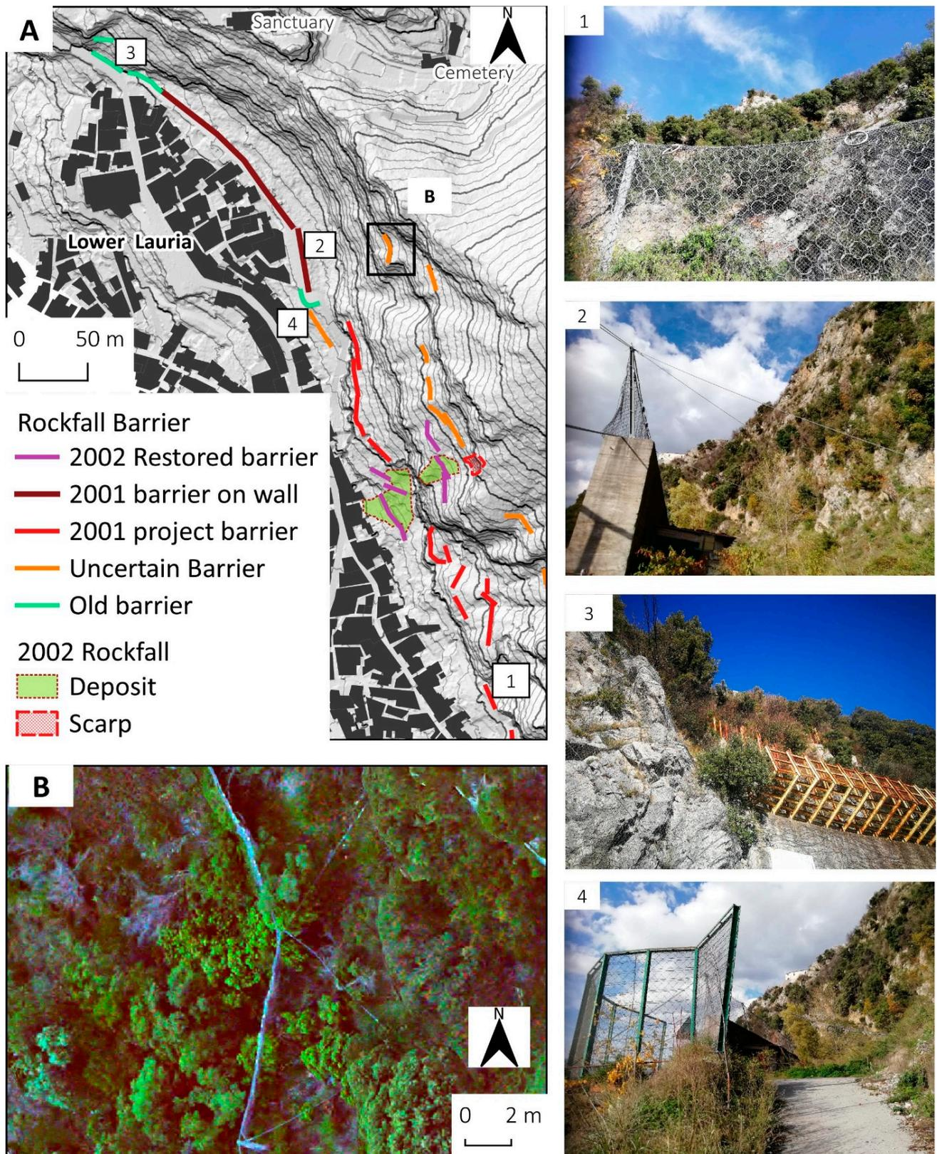
**Figure 4.** Example of digitized and geocoded rockfall barriers. **(A)** Classification of the barriers with the location of some representative photos (taken in February 2020 field survey). Photo 1 shows a certified rockfall barrier of 2001. Photo 2 shows a 1500 kJ barrier installed over a wall. Photos 3 and 4 show an old barrier (pre-2001) without documentation. **(B)** Barrier of uncertain age detected with UAV LiDAR and orthophoto (details in Figure 7).
