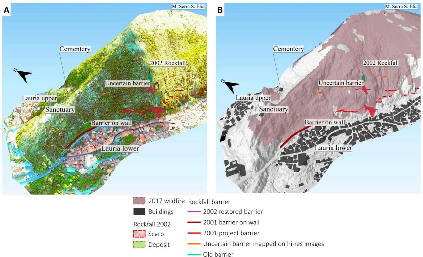
**Figure 8.** Exported 3-D view of the study area based on DTM LiDAR with rockfall barriers overlapped, obtained with the Qgis2threejs plugin [29]. (A) 3-D view with overlapped orthophoto. (B) 3-D view with overlapped shaded relief and burnt area. The 3-D views are available on the Zenodo platform [50].
