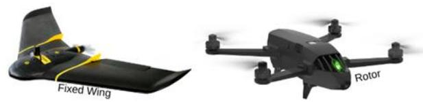
**Figure 1.** The fixed-wing eBee Sequoia (SQ) and the Parrot Anafi rotor drones from Parrot Group: picture concept adopted and modified from [1].
