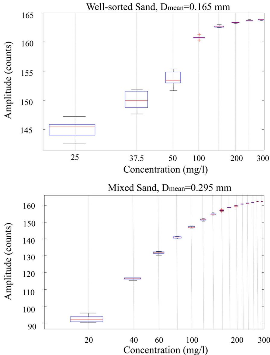
**Figure 3.** Raw backscatter amplitude vs. concentration for two experiments with well-sorted (**top panel**) and mixed (**lower panel**) sand samples. Each case was repeated six times for each tested concentration (the central mark is median, the edges of each box are the 25th and 75th percentiles, and the whiskers show extremes).
