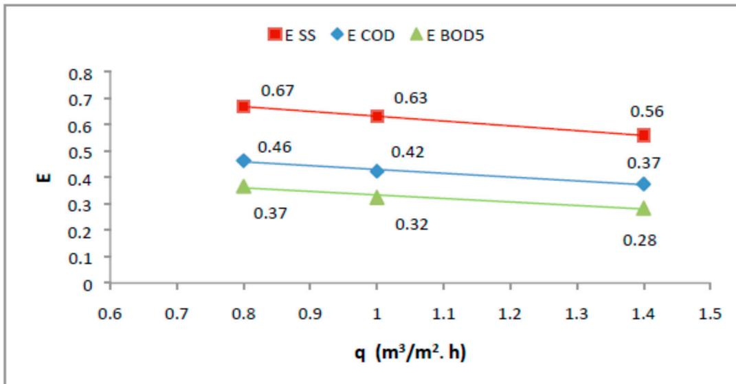
Figure 3. Effect of q on SS, COD and BOD<sub>5</sub> Efficiency.
