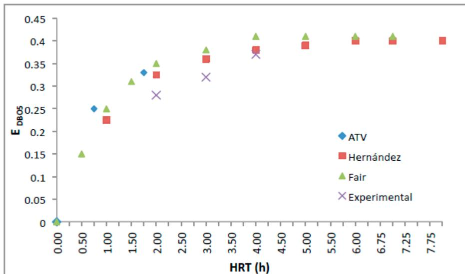
Figure 6. Effect of HRT on BOD<sub>5</sub> Efficiency.
