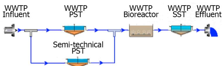
Figure 1. Semi-technical PST: schematic diagram of the process.
