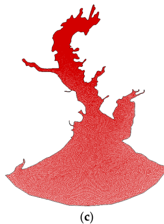
Figure 1. (a) Location of Tieshangang Bay; (b) Topographic map of Tieshangang Bay; and (c) the unstructured grid for the MIKE 21 FM and a close-up of the variable mesh resolution.
