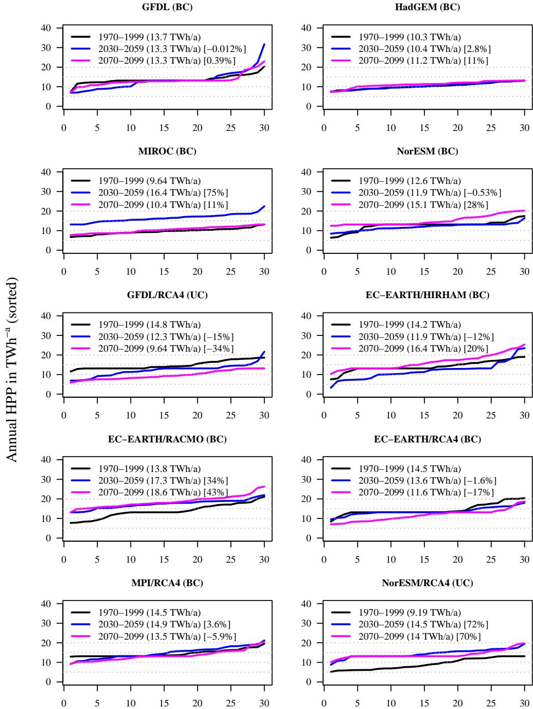
Figure S 7: Sorted annual HPP in  $TWh^{-a}$  of the three 30-years periods and operation scenario hpp\_1500MW\_01a (low seepage rate), in brackets the mean annual production and in square brackets the change signal
