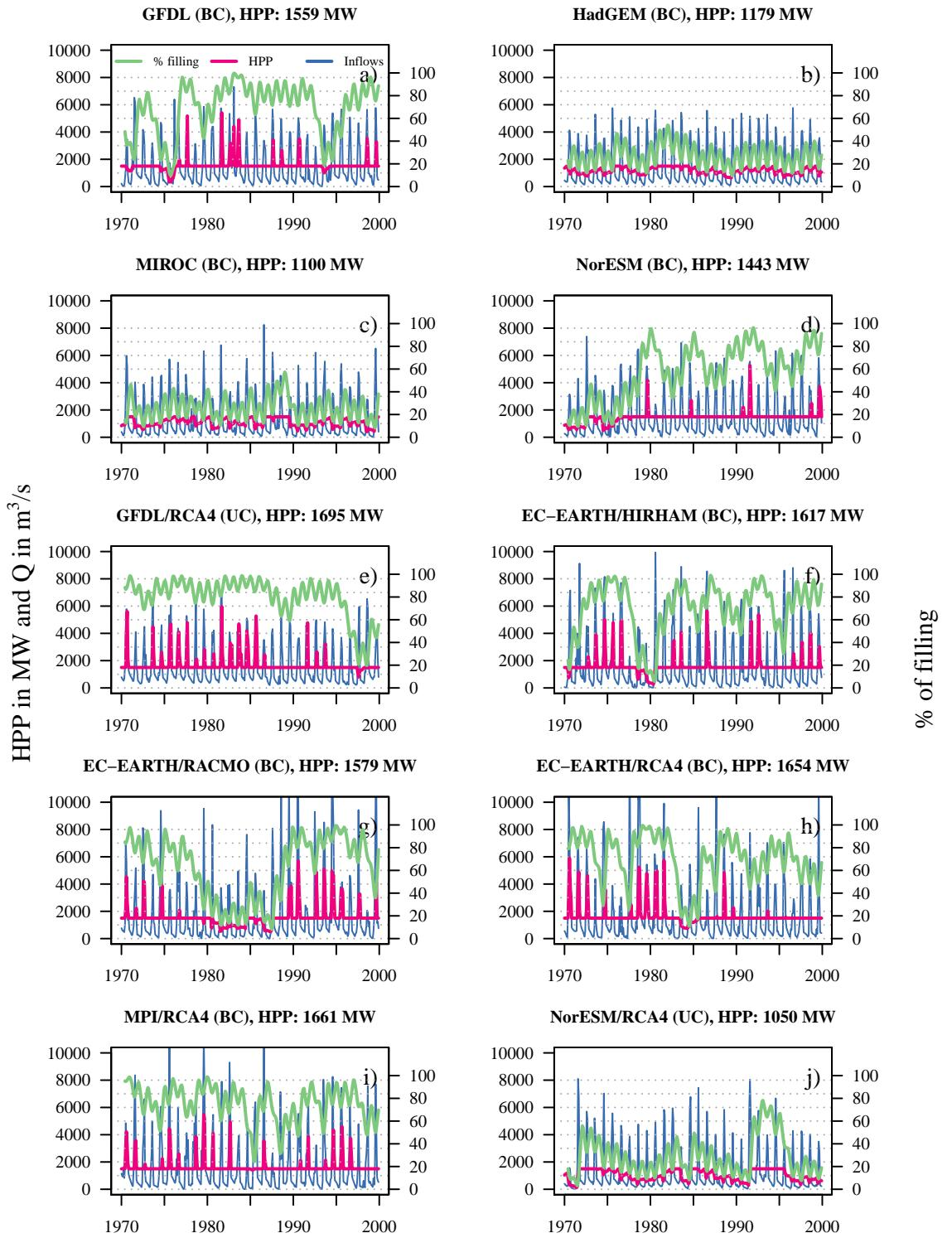
Figure S 3: Reservoir filling, inflows, and HPP simulated with climate model input in the reference period and operation scenario hpp\_1500MW\_01a (low seepage rate)
