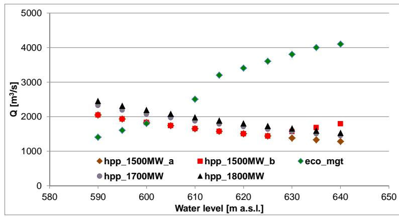
Figure S 1: GERD rule curves of the different operation scenarios
