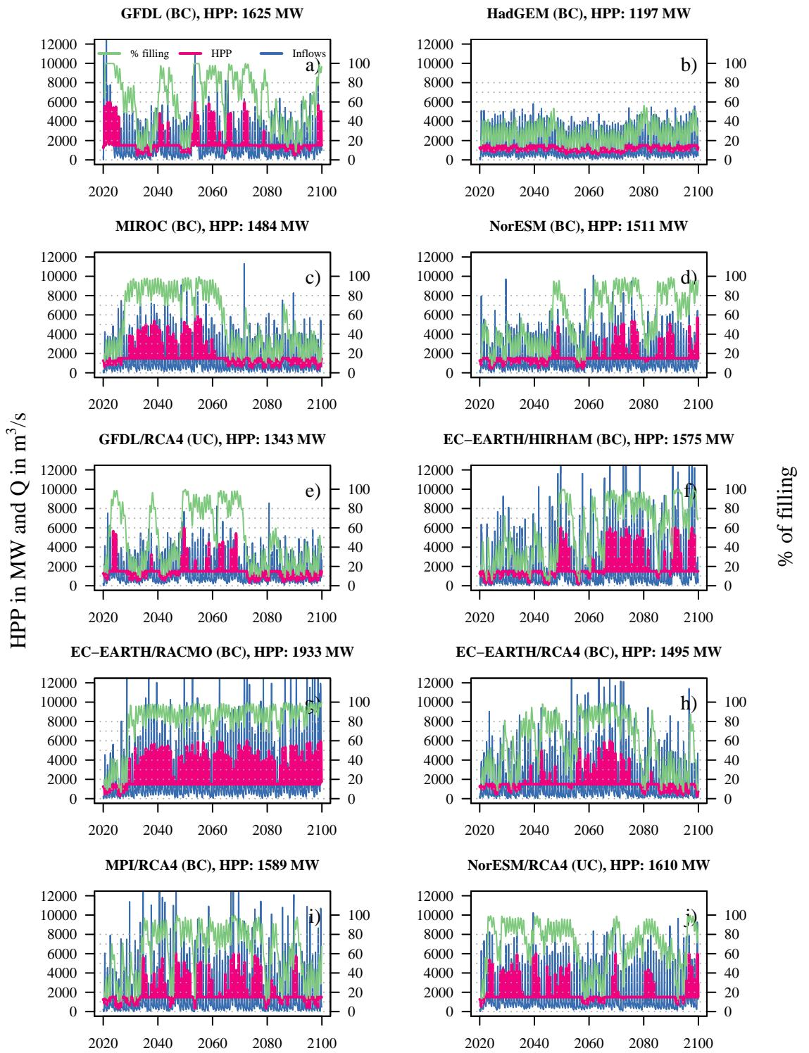
Figure S 6: Operation scenarios under climate change projections and operation scenario hpp\_1500MW\_01a (low seepage rate)
