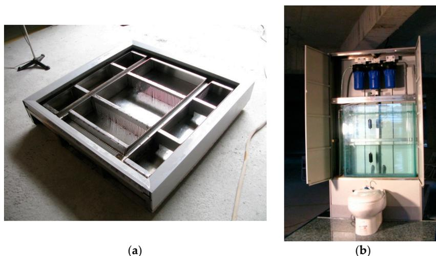
**Figure 3.** Prototype model of greywater processing: (a) Primary filtration and sedimentation; (b) Filtration, sterilization and water storage.
