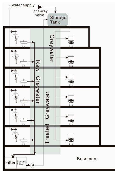
Figure 1. Conventional Greywater System.
