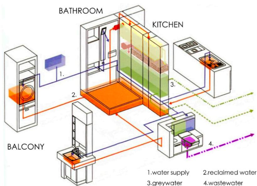
**Figure 2.** Conceptual diagram of Interior Customized Greywater System (ICGS).
