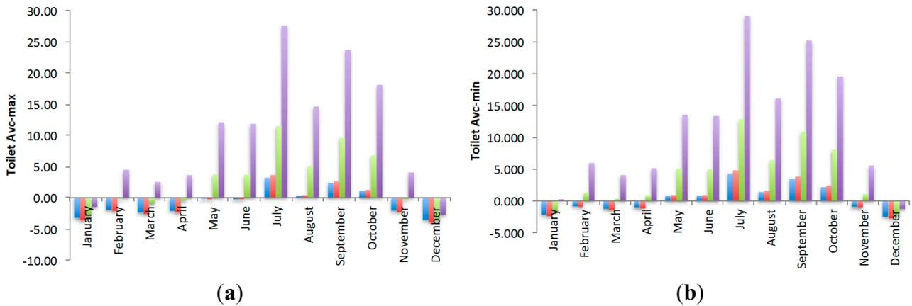
**Figure 5.** Monthly balance of rainwater per household type (available water ( $Wa$ ) in m<sup>3</sup>/month) after flush toilet (a) Toilet,  $A_{vc_{max}}$ ; (b) Toilet,  $A_{vc_{min}}$  blue:  $Hra = 45$  m<sup>2</sup>; red:  $Hra = 50$  m<sup>2</sup>; green:  $Hra = 100$  m<sup>2</sup>; purple:  $Hra = 200$  m<sup>2</sup>).
