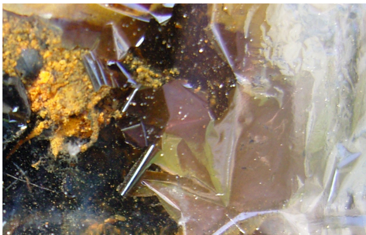
Figure F1. Corrosion features associated with fibrous (0.1 mm diameter) \text{Fe}^0 in saline water [PS14], photographed following conclusion of the desalination trial. Black = water filled porosity. Orange/yellow spheroids = hydrated \beta\text{-FeOOH}\cdot m\text{H}_2\text{O} ( \text{Fe}^{3+}\text{O}(\text{O}, \text{Cl}) ) formed by precipitation of \text{Fe}^{3+} ions in the water. Dark grey nodules surrounded by orange spheroids = bog iron ( \text{Fe}_3\text{O}_4 , magnetite). Off white to green and purple sheets growing into the water from the bright white rods = mixed valance green rust complex ( \text{Na}^I_{(a=1-c-b)}\text{Fe}^{II}_{(b=1-c-a)}\text{Fe}^{III}_c(\text{OH})_2]^{x-}\cdot[(x/n)\text{Cl}^{n-}\cdot m\text{H}_2\text{O}]^{x+} , where a + b + c = 1 ) formed from the accretion of \text{Fe}^{2+} and \text{Fe}^{3+} ions in the water. The bright white rods of \text{Fe}(\text{OH})_2 pseudomorph after and surround a \text{Fe}^0 core. They are the initial corrosion product. They are initially replaced at the water interface by purple, \beta\text{-FeOOH} . These act as a template for green rusts ( \text{Na}^I_{(a=1-c-b)}\text{Fe}^{II}_{(b=1-c-a)}\text{Fe}^{III}_c(\text{OH})_2]^{x-}\cdot[(x/n)\text{Cl}^{n-}\cdot m\text{H}_2\text{O}]^{x+} , where a + b + c = 1 ) sheets. The green rusts are gradually replaced by ( \beta\text{-Fe}^{3+}\text{O}(\text{O}, \text{Cl})\cdot n\text{H}_2\text{O} ). The increase in the proportion of \text{Fe}^{III} species is initially signified by a rusty purple color which is then replaced by a yellow color when the precipitate is dominated by highly hydrated \text{FeOOH}\cdot m\text{H}_2\text{O} . The purple \text{FeOOH} becomes increasingly yellow in color with increased hydration. Fe corrosion species in this photograph have been identified by their color and morphology. The left edge (centre) of the photograph truncates a trapped hydrogen gas bubble. The formation of the grey precipitate is associated with the upper surface of the gas bubble. Field of view = 2 cm. The common colors of the various \text{Fe}_2\text{O}_3 , \text{Fe}_3\text{O}_4 corrosion species are: (i) hematite = red; (ii) maghemite = reddish brown; (iii) magnetite = black; (iv) goethite = yellow brown; (v) = lepidocrocite = orange; (vi) ferrihydrite = red-brown; (vii) akaganeite = purple to red brown/purple to orange/yellow; (viii) layered double hydroxides (white and green rusts) = white to green. The purple colour indicates the incorporation of \text{Na}^+ (see Appendix H).
