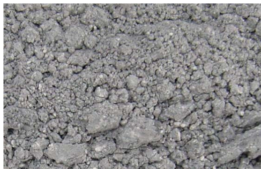
Figure 3. ZVM TPA powder used in the initial commercial trials (E145, E146, Tables C5–C12 and D3), prior to placement in the cartridges. Field of view = 2 cm.
