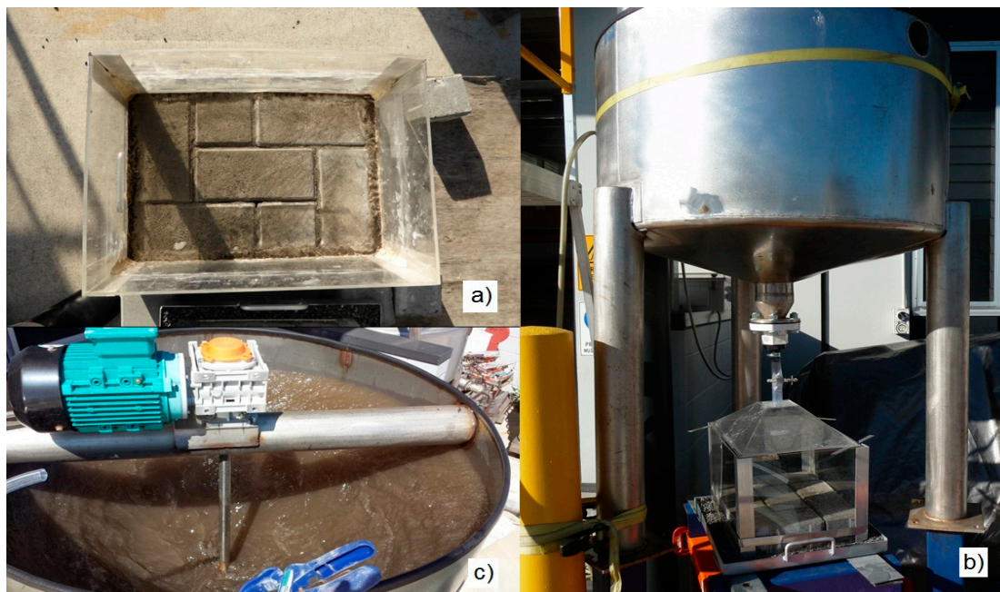
Figure 5. Accelerated stormwater simulation testing setup. (a) Paver test model; (b) Test rig; (c) Tank stirrer.
