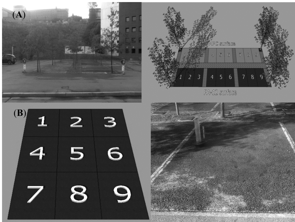
Figure 1. (A) Scheme of the eighteen car parking bays analyzed; and (B) measurement zones selected within each car park bay and LCS on-site.
