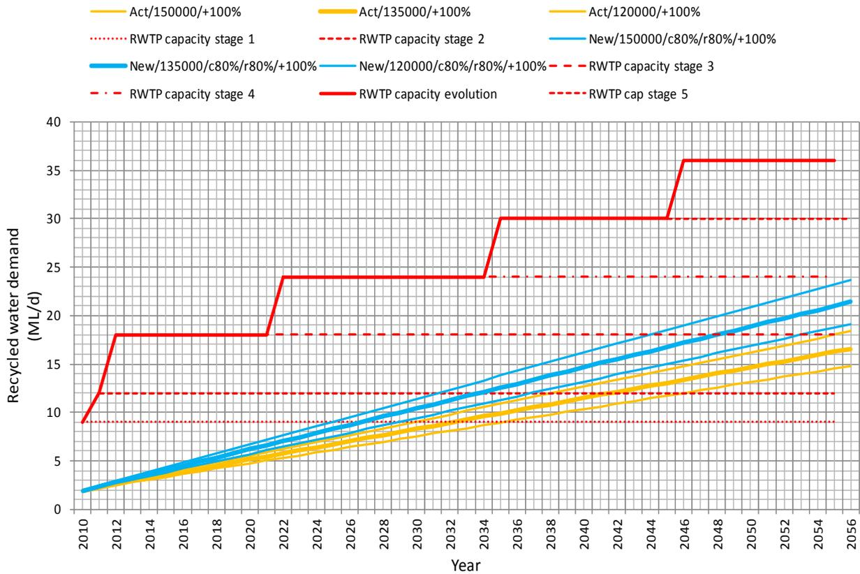
Increasing the peak factor to 2.3, Figure 4 is obtained. For this higher peak demand factor considered, one more stage would be needed for both schemes: in the worst case scenarios for the proposed scheme, the stage 5 limit (30 ML/d) would be approached, but not exceeded. For the present scheme design, stage 4 RWTP capacity (24 ML/d) would be adequate even for the worst case.
