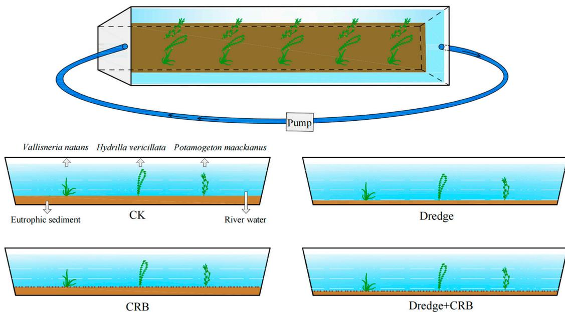
**Figure 1.** Schematic diagram of the experimental device and experimental design. CK: control group; Dredge: dredging treatment group; CRB: calcium-loaded clay granular inactivating treatment group; Dredge + CRB: combined dredging and CRB treatment group.
