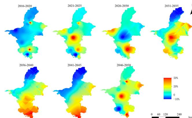
**Figure 14.** Changes in  $R(t)$  value of potential impact level of check dams in Ningxia region under RCP8.5 scenario.
