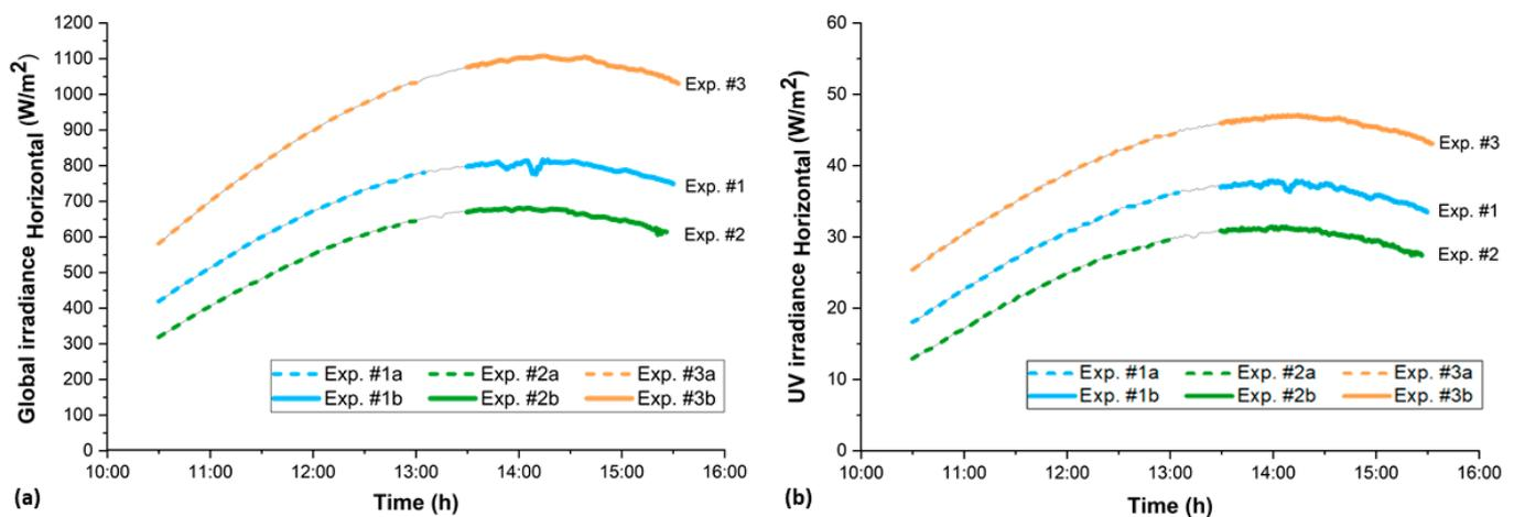
**Figure 2.** Climatic conditions of global irradiance (a) and UV irradiance (b) versus solar exposure time of experiments #1, #2 and #3 performed on the rooftop of the E.P.S. of Linares (Jaén, Spain).
