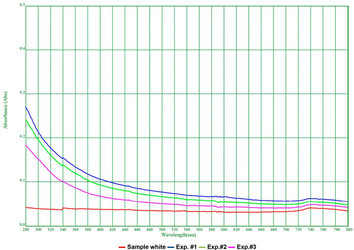
**Figure A2.** Absorbance (UV-Vis wavelength range) of the samples of the secondary effluent wastewater from the Linares WWTP (Jaén, Spain) used in the experimental trials #1, #2, and #3, with a respective initial turbidity of 7.77 NTU, 7.70 NTU, and 7.64 NTU. The white sample was created using ultrapure water (Milli-Q). Quartz cuvettes were used.
