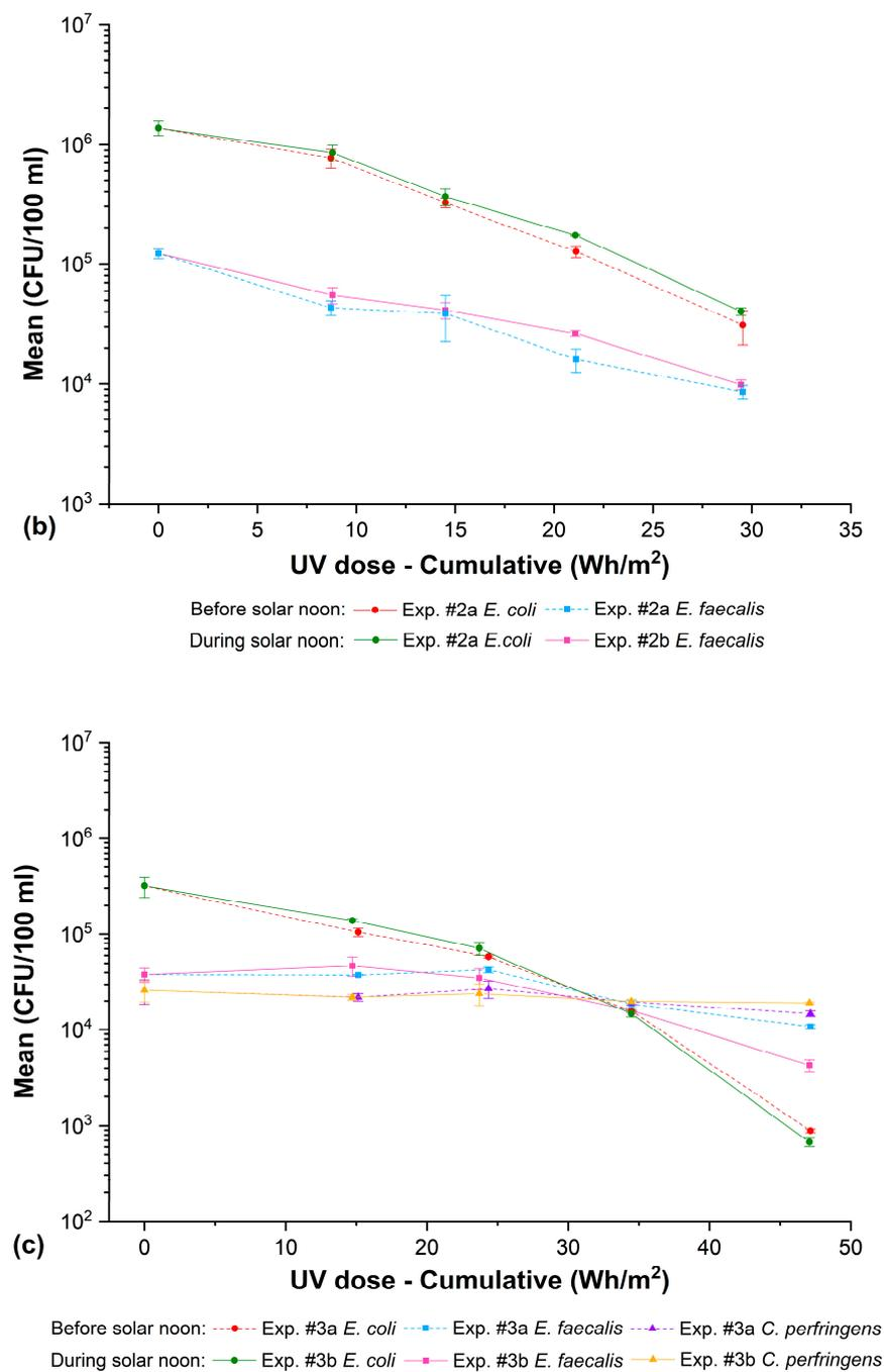
**Figure 4.** SODIS disinfection kinetics for *E. coli*, *E. faecalis*, and *C. perfringens* during tests #1 (a), #2 (b), and #3 (c), before solar noon and during solar noon, with controlled temperature (<20 °C). The reciprocity law was valid for *E. coli* and underwent deviations for *E. faecalis*. *C. perfringens* showed no significant results. The detection limit (100 CFU/100 mL) was not reached in any test.
