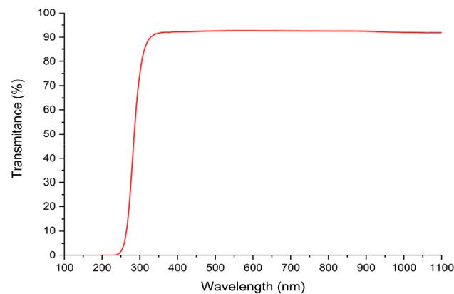
**Figure A1.** UV-Vis transmission spectrum of borosilicate glass. This material allows for a high transmittance of the UV spectrum (UVA-UVB), being able to reach 90% of the visible spectrum and the infrared spectrum.
