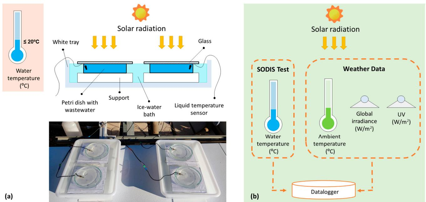
**Figure 1.** Experimental setup: (a) Scheme of solar disinfection during the experimental trials and (b) scheme of control and recording of climatic conditions and water sample temperature.
