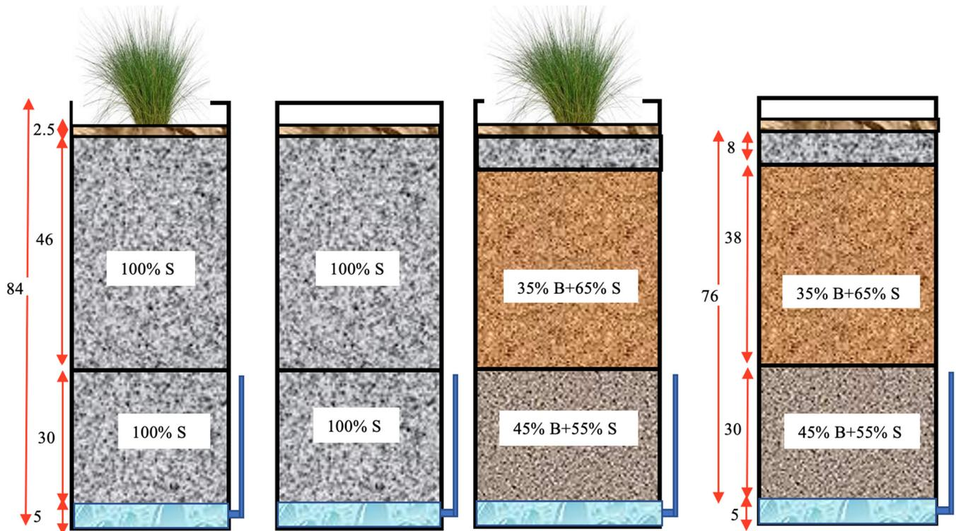
**Figure 1.** Schematic diagrams of (left to right) sand-modified bioretention cell with plants (S+P), sand-modified bioretention cell (S), biochar-amended modified bioretention cell with plants (BC+P), and biochar-amended modified bioretention cell (BC). Units are in cm.
