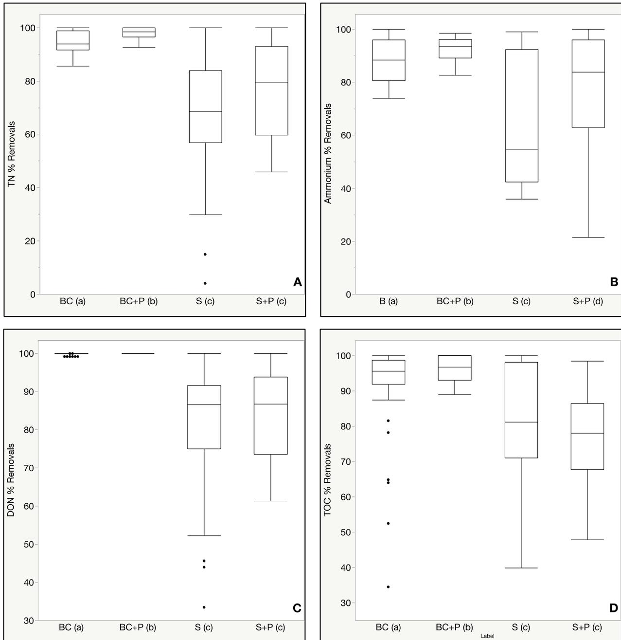
**Figure 3.** Box and whisker plots of N-species and TOC removal efficiencies for events 1–7: (A) TN, (B) ammonium ( $\text{NH}_4^+$ ), (C) DON, and (D) TOC. Labels with different letters show statistically significant differences in mass removals.
