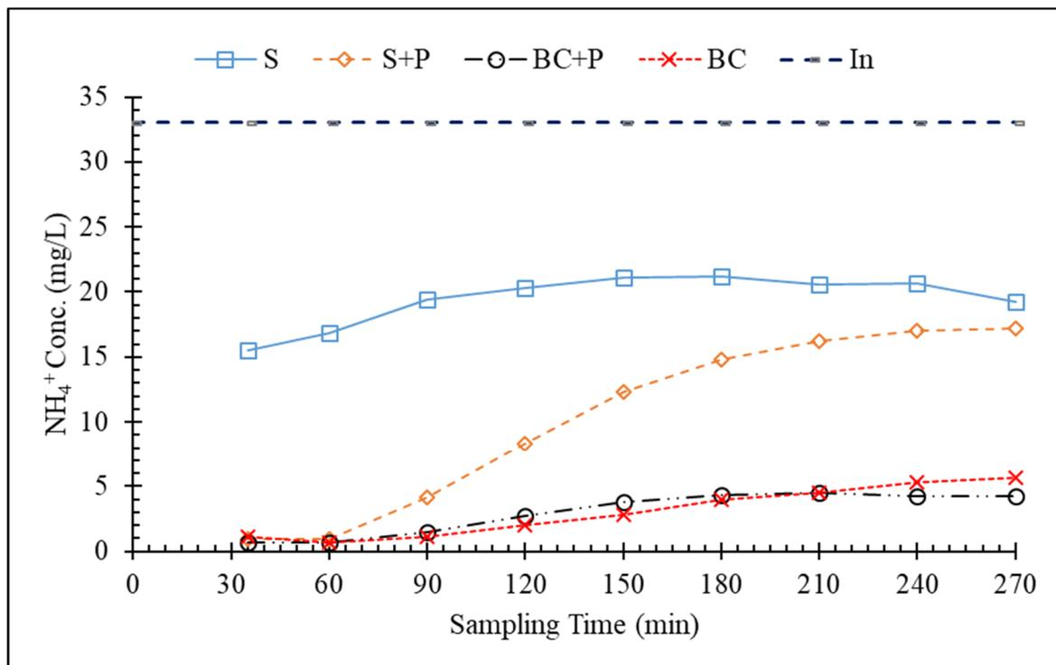
**Figure 5.** Pollutant breakthrough curve for NH<sub>4</sub><sup>+</sup> for four modified bioretention systems during Event 5.
