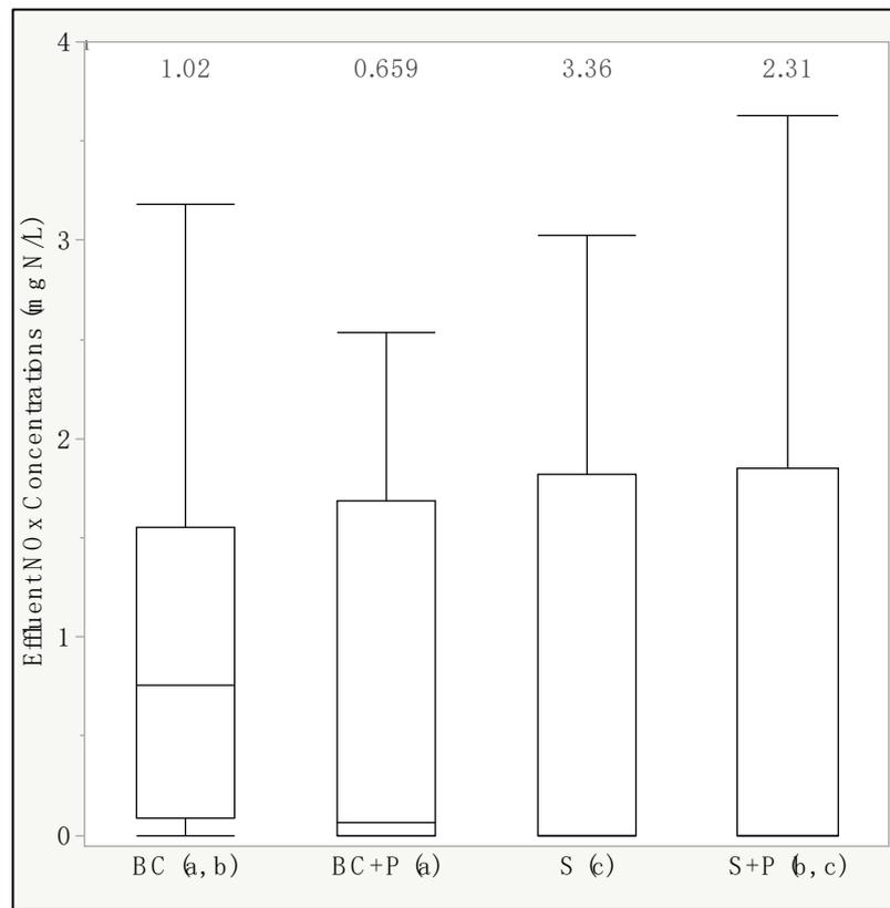
**Figure 4.** Effluent NO<sub>x</sub> concentrations for Events 1–7 (outliers excluded). Mean values are displayed above each box. Labels with different letters represent statistically significant differences in effluent concentrations.
