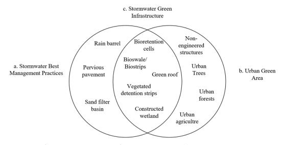
Figure 1. Defining stormwater green infrastructure practices. (a) Stormwater Best Management Practices are engineered practices, including both green and non-green components. (b) Urban Green Area includes both engineered and non-engineered practices that have green components. (c) Stormwater green infrastructure is at the intersection of these and includes engineered practices with green components.
