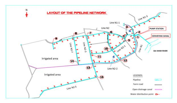
**Figure 2.** Layout of the pipeline network of Thanh Nghia irrigation system (Numbers 1–15 are of water intake positions).
