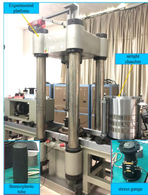
**Figure 4.** Experimental instrument.
