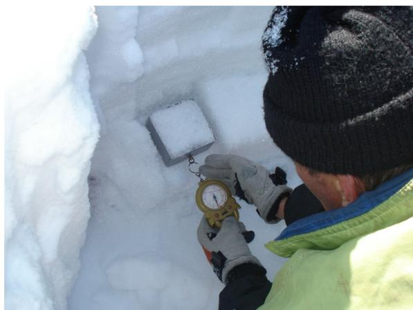
**Figure 2.** Measuring the shear strength of snow in a weak layer.
