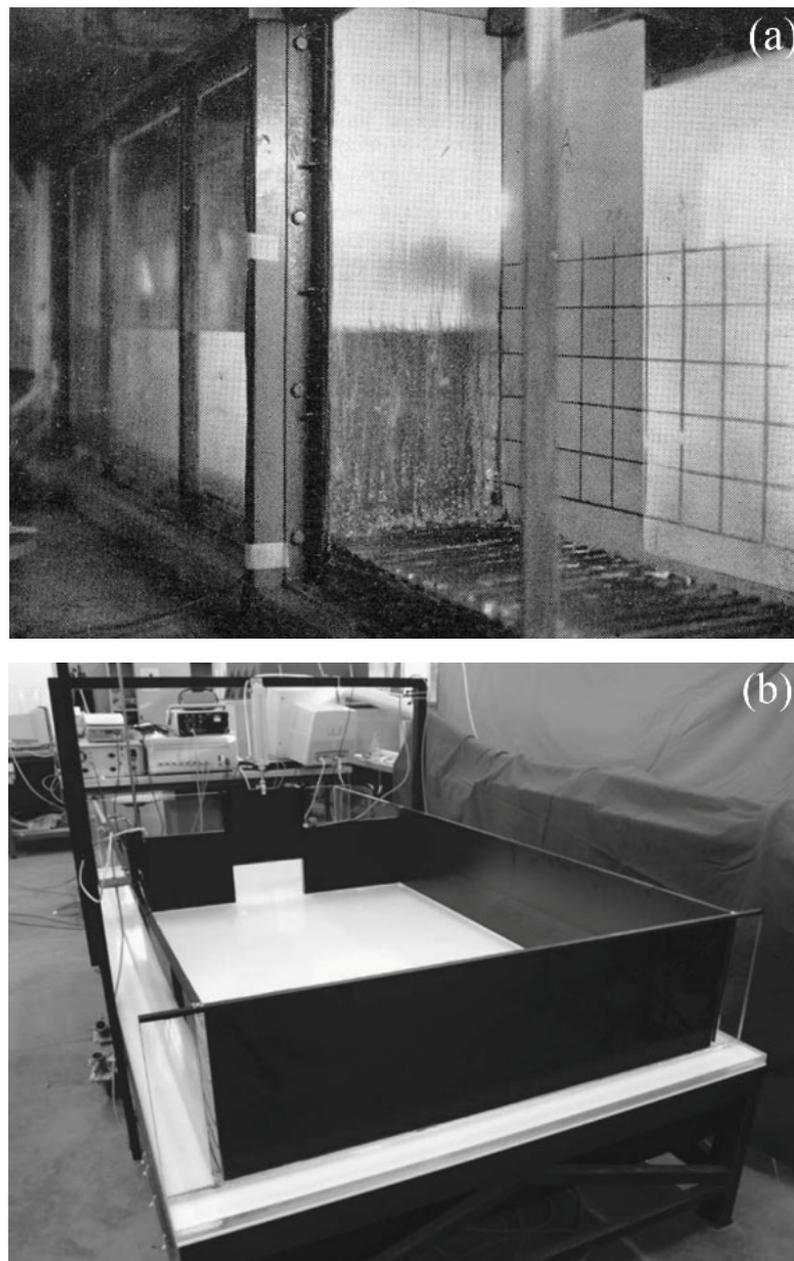
**Figure 1.** Pictures of typical experimental facilities for dam-break flow investigations. (a) Total dam-break in a rectangular channel (reprinted with permission from Ref. [13]; courtesy of International Association of Hydrological Sciences). (b) Prismatic tank for partial dam-break experiments (reprinted with permission from Ref. [14]).
