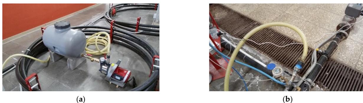
**Figure 3.** Installation of the pump-reservoir system (a) and connection to the node (b).
