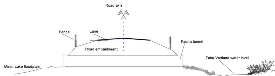
**Figure 2.** Schematic cross section of BR-471 crossing ESEC-Taim including the representation of fauna tunnel and fences.
