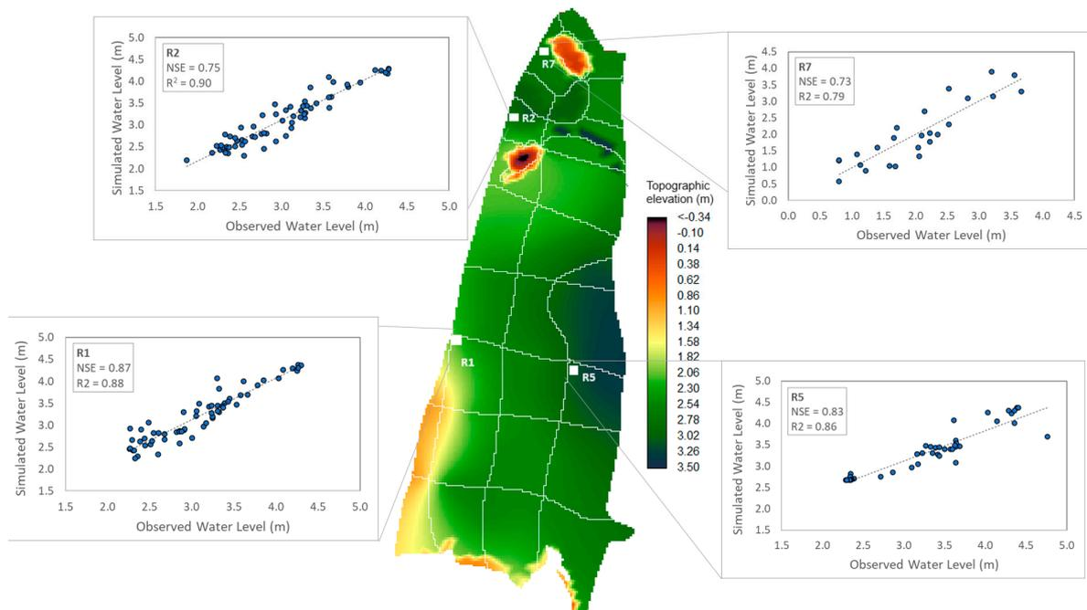
**Figure 3.** Scatter plots for the four representative water level stage stations within Taim Wetland—white lines in the Taim area indicate the cells of the model over the topographic elevation.
