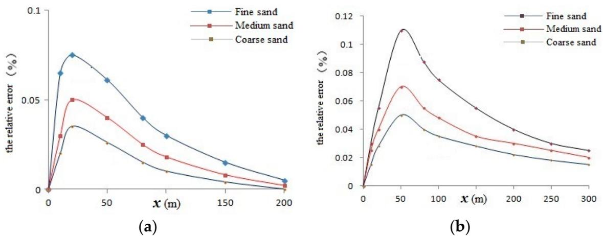
**Figure 3.** Relative error between the analytical and numerical solutions of the phreatic water level. (a)  $t = 24$  h. (b)  $t = 48$  h.
