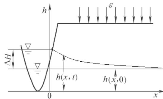
Figure 1. Seepage field near a river channel.
