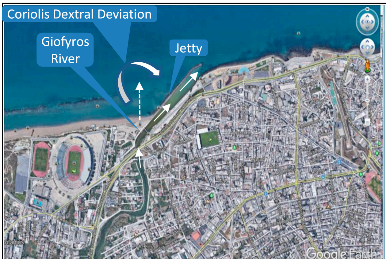
Figure 8. The jetty for a Coriolis dextral deviation of the Giofyros mouth.
