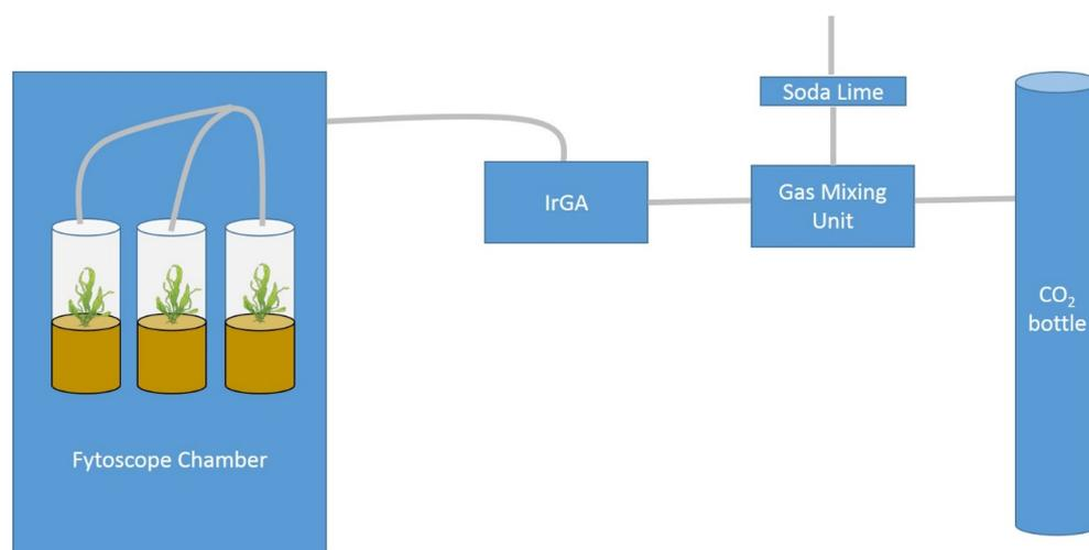
**Figure 1.** Schematics of the  $\text{CO}_2$  enrichment incubation system, consisting of a gas mixing unit regulated using an Infra-red Gas Analyser (IrGA) connected to a  $\text{CO}_2$  bottle and a soda lime cylinder to remove any ambient  $\text{CO}_2$ , precisely recording the  $\text{CO}_2$  levels in the mesocosms.
