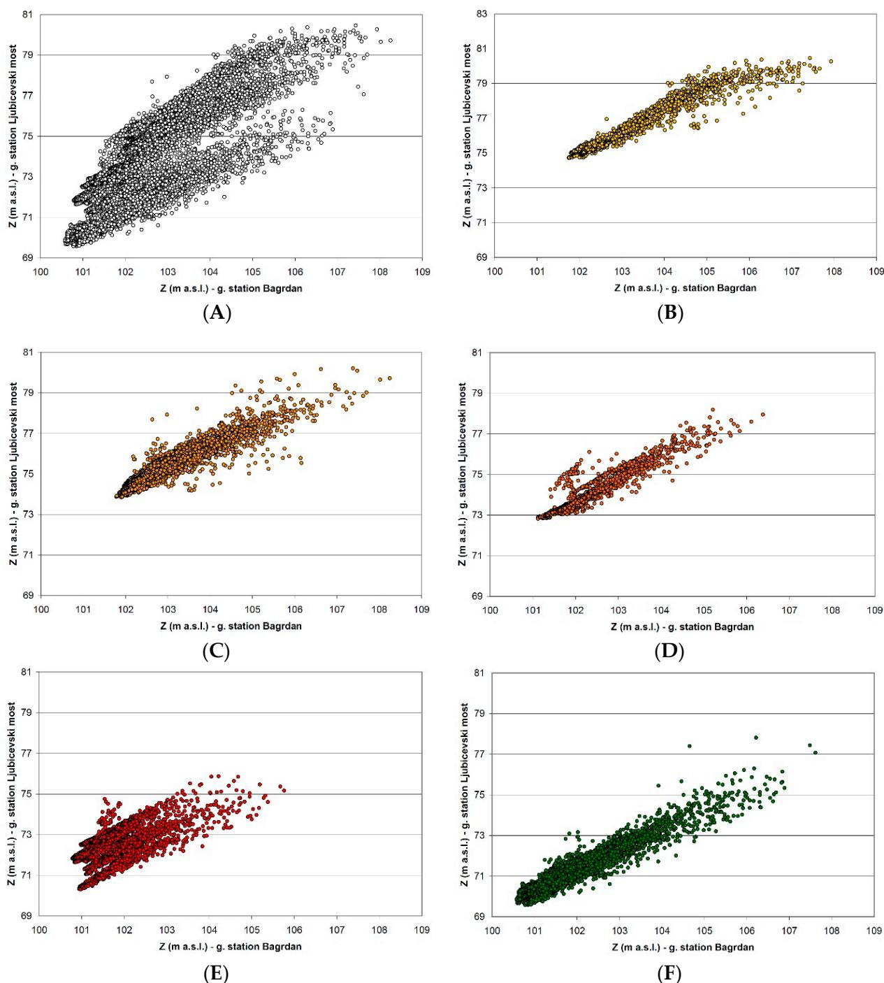
**Figure 8.** Water levels of the Velika Morava River at Ljubičevski Most vs. Bagrdan: (A)—total period, (B) 1952–1962, (C) 1963–1981, (D) 1982–1989, (E) 1990–1999, and (F) 2000–2018.
