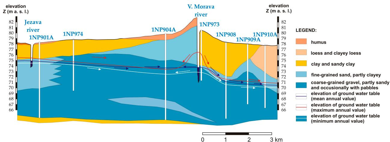
**Figure 10.** Hydrogeological section at the Ljubičevski Most gauging station, including observation wells on the left and right banks. Groundwater levels reflect the calculated annual averages for 1988 (dark blue line) and extreme situations (flood discharges red line and dry period white line).
