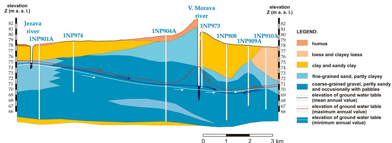
**Figure 11.** Hydrogeological section at the Ljubičevski Most gauging station, including observation wells on the left and right banks. Groundwater levels reflect the calculated annual averages for 2008 (dark blue line) and extreme situations (flood discharges red line and dry period white line).
