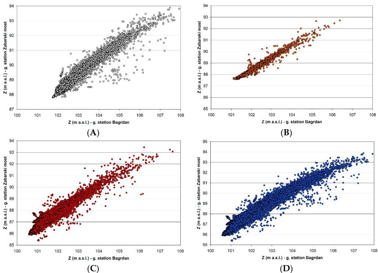
**Figure 9.** Water levels of the Velika Morava River at Bagrdan vs. Žabarski Most: (A)—total period, (B) 1952–1981, (C) 1982–1989, and (D) 1990–2018.
