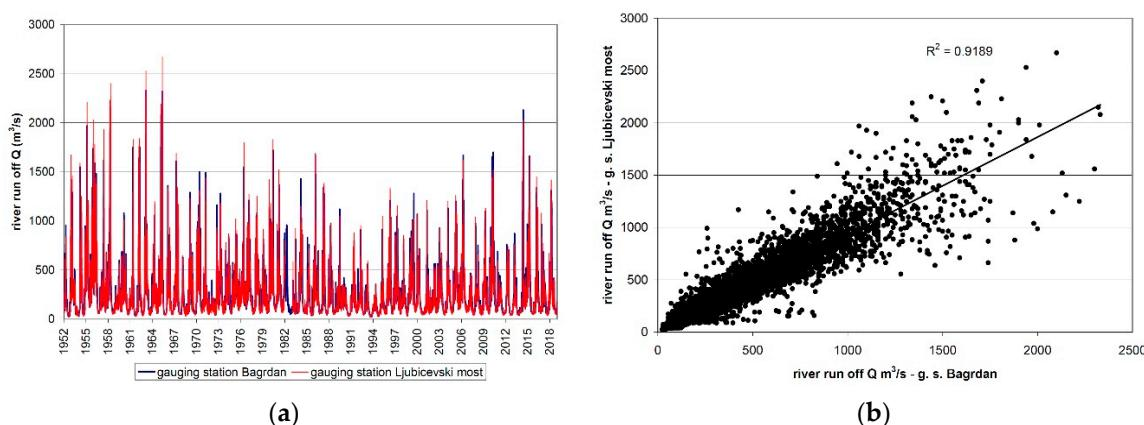
**Figure 3.** (a) Hydrographs of the Vélika Morava River at Ljubičevski Most and Bagrdan from 1952 to 2018; and (b) correlation between discharges observed at Ljubičevski Most and Bagrdan (1952–2018).
