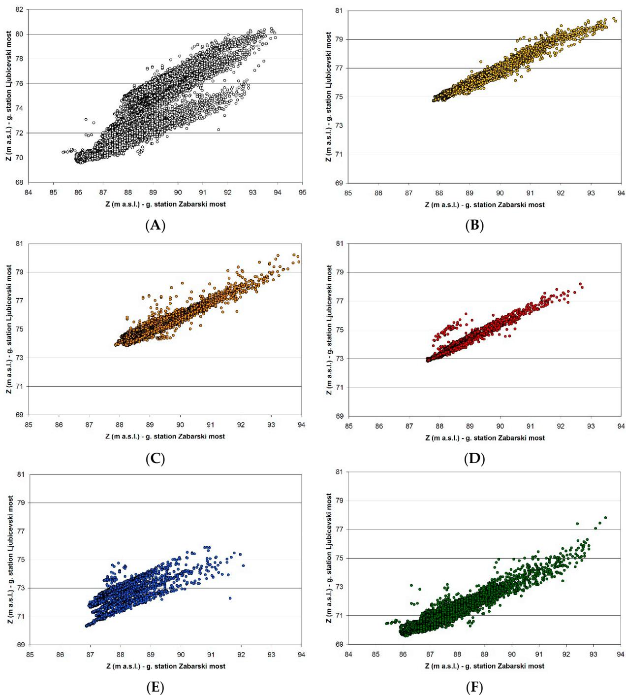
**Figure 7.** Water levels of the Velika Morava River at Ljubičevski Most vs. Žabarski Most: (A)—total period, (B) 1952–1962, (C) 1963–1981, (D) 1982–1989, (E) 1990–1999, and (F) 2000–2018.
