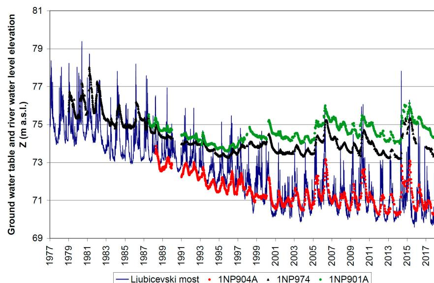
**Figure 5.** Velika Morava River water levels at Ljubičevski Most and groundwater levels at the observation wells on the left bank (1977–2018).
