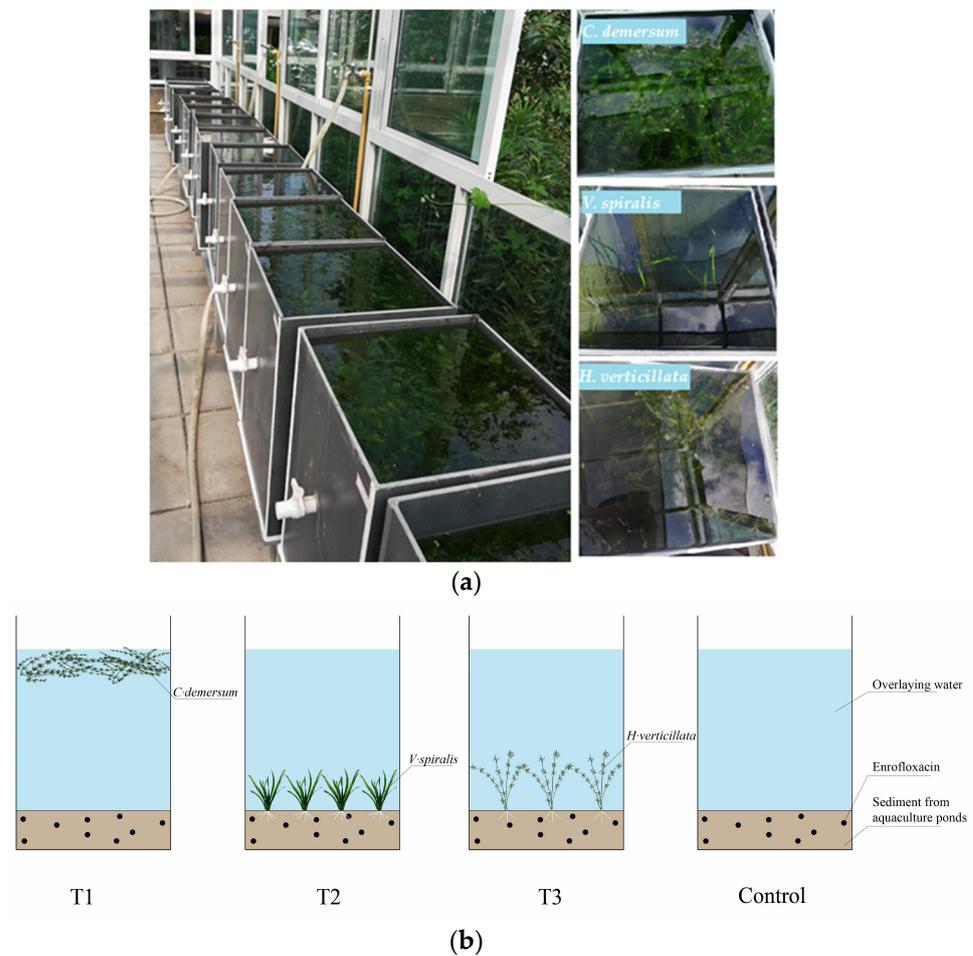
**Figure 1.** (a) The experimental images. (b) Schematic of the experimental set-up.
