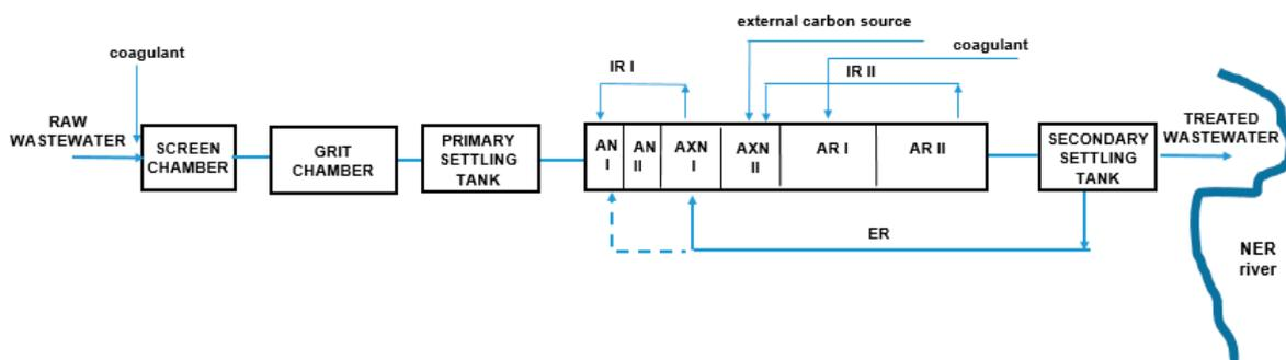
**Figure 3.** Scheme of the GWWTWP technological system (for one process line). AN—anaerobic chamber, AR—aerobic chamber, AXN—anoxic chamber, IR—internal recirculation, ER—external recirculation.
