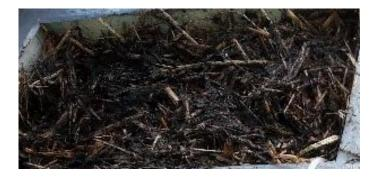
Figure 3. View of the compost after 15 days of composting (straw:sewage sludge:fly ash—1:10:1).
