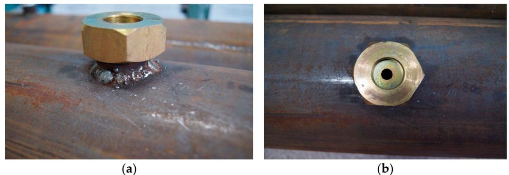
**Figure 3.** Method of fixing discs on the pipeline: (a) side view, (b) top view.
