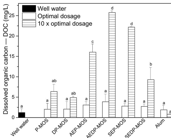
**Figure 6.** Dissolved organic carbon (DOC) variation as a function of *Moringa oleifera* seed-derived and alum coagulants dosages (optimal dosage and 10× optimal dosage) in jar tests after coagulation, flocculation, and sedimentation. Bars with the same letter represent means that did not differ significantly ( $p \leq 0.05$ ) based on Tukey HSD post hoc test.
