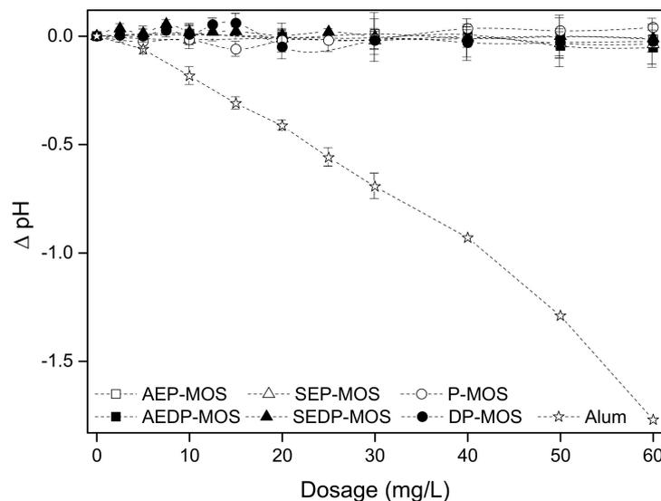
**Figure 4.** pH variation as a function of *Moringa oleifera* seed-derived and alum coagulants dosages in jar tests after coagulation, flocculation, and sedimentation. Initial pH was  $7.10 \pm 0.12$ .
