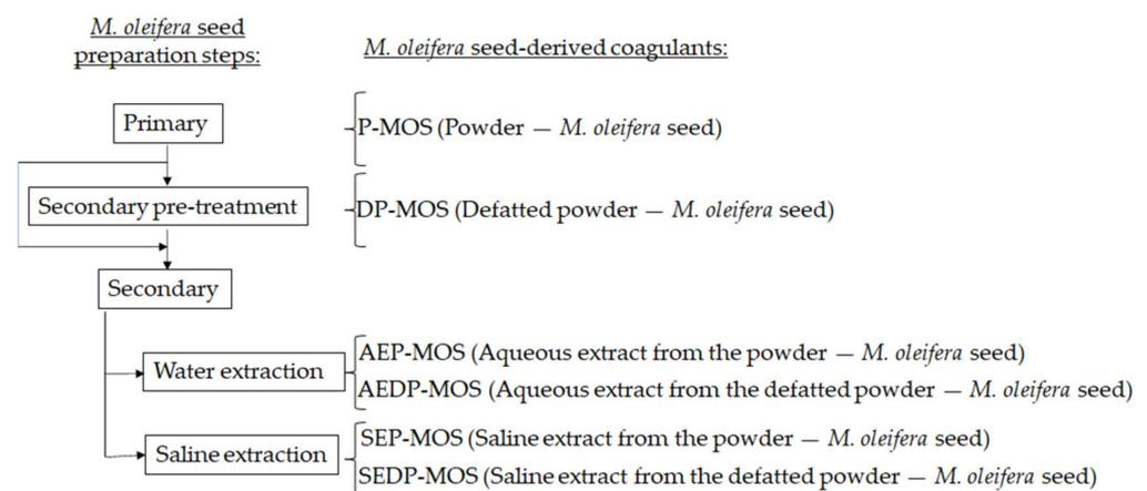
**Figure 1.** Processing steps for the production of *M. oleifera* seed-derived coagulants.
