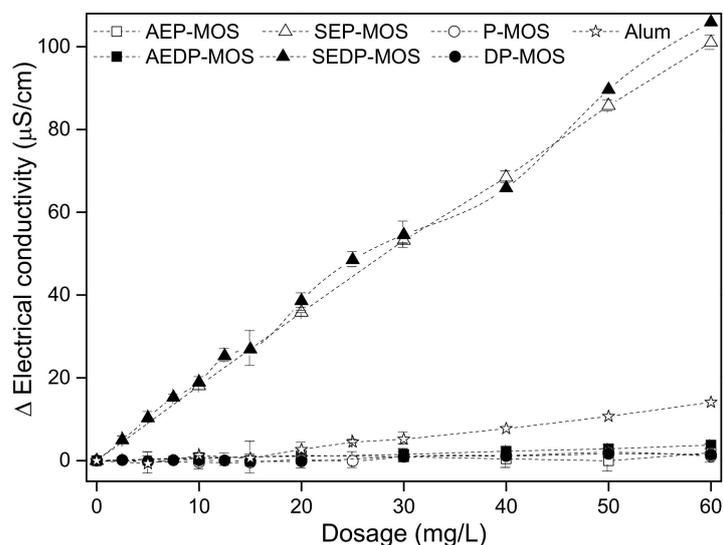
**Figure 5.** Electrical conductivity variation as a function of *Moringa oleifera* seed-derived and alum coagulants dosages in jar tests after coagulation, flocculation, and sedimentation. Initial conductivity was  $49.1 \pm 4.4 \mu\text{S}/\text{cm}$ .
