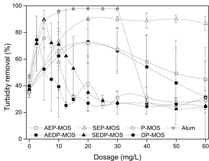
**Figure 2.** Turbidity removal (%) as a function of *Moringa oleifera* seed-derived and alum coagulants dosages in jar tests after coagulation, flocculation, and sedimentation. Initial turbidity was  $200.8 \pm 9.3$  NTU.
