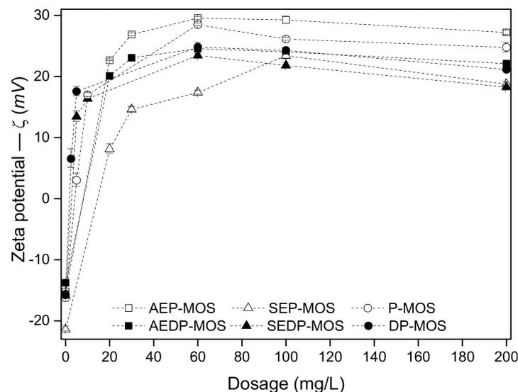
**Figure 3.** Zeta potential (mV) as a function of *Moringa oleifera* seed-derived coagulants dosages in jar tests.
