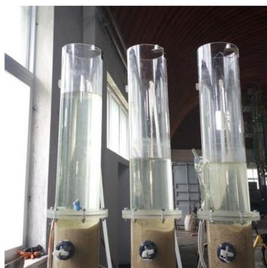
**Figure 4.** Photos of equipment in operation; SSF1<sup>#</sup>, SSF2<sup>#</sup>, and SSF3<sup>#</sup> (from left to right). Clogging became evident in SSF1<sup>#</sup>.
