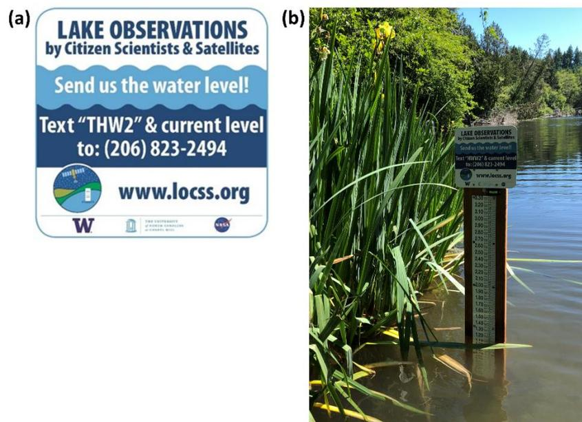
**Figure 2.** An example of a LOCSS lake gauge with a sign on top for texting in measurements. Figure (a) depicts a LOCSS lake gauge sign and what a citizen scientist would read. Figure (b) depicts a LOCSS lake gauge located in Lake Howard, WA.
