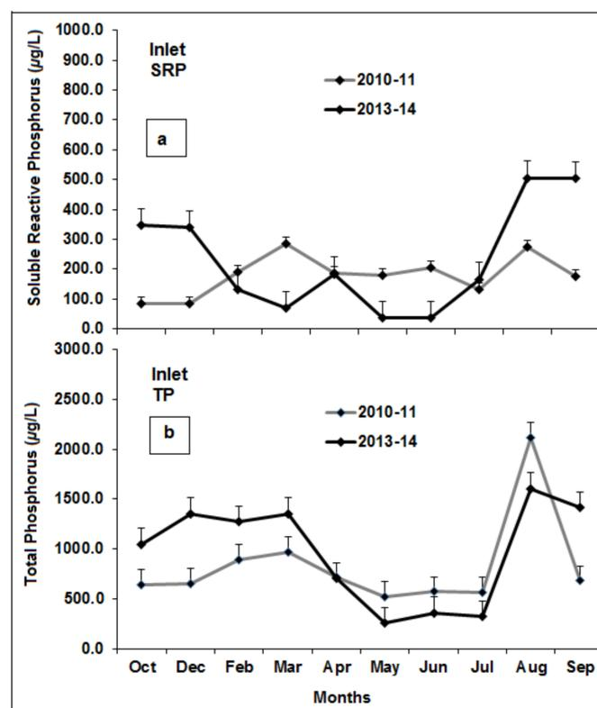
**Figure 10.** Soluble reactive phosphorus (SRP) and total phosphorus (TP) concentrations ( $\mu\text{g/L}$ ) measured at combined inlet near Magüayo for common sampling dates during (a) 2010–2011 and (b) 2013–2014.
