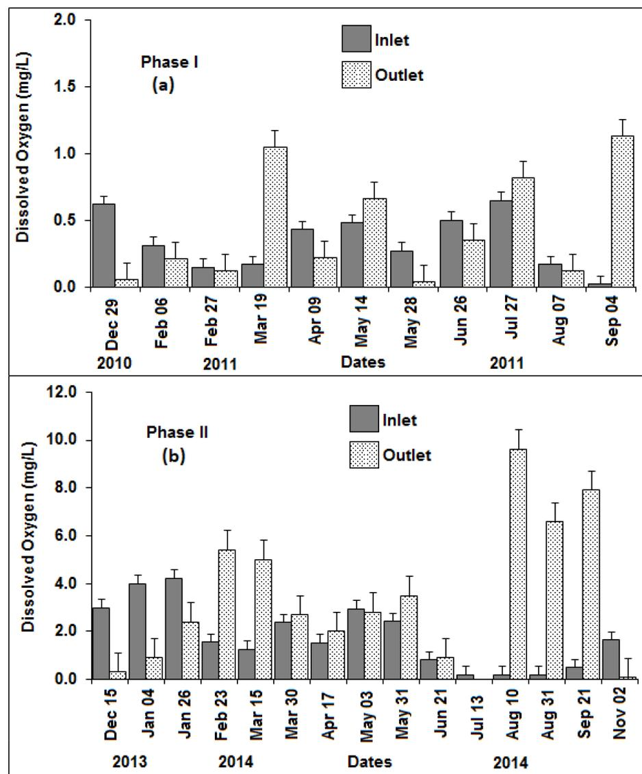
**Figure 5.** Dissolved oxygen (DO) from combined inlet and the lagoon’s outlet for the period of: (a) 29 December 2010 to 4 September 2011 (Phase One) and (b) 15 December 2013 to 2 November 2014 (Phase Two).
