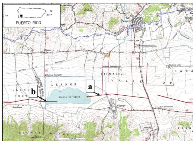
**Figure 1.** Location of Laguna Cartagena (USGS (US Geological Survey) San German Quadrangle). The shaded area denotes the water surface level (the 10 m contour) at the time of the 1982 update. (a) Inlet to the lagoon (combined inlet canal, the Principal Drainage Canal adjacent to the town of Magüayo and (b) the outlet (exit canal) within the lagoon. The dashed blue line indicates the jurisdictional limits of the National Wildlife Refuge around the lagoon.
