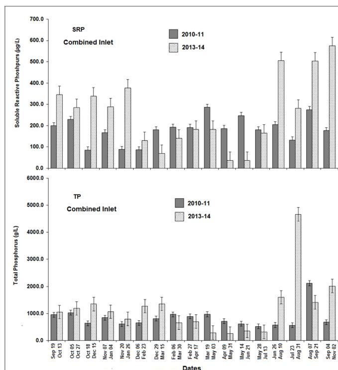
**Figure 8.** Soluble reactive phosphorus (SRP) and total phosphorus (TP) concentrations ( $\mu\text{g/L}$ ) measured at the combined inlet from 19 August 2010 to 4 September 2011 and from 13 October 2013 to 2 November 2014.
