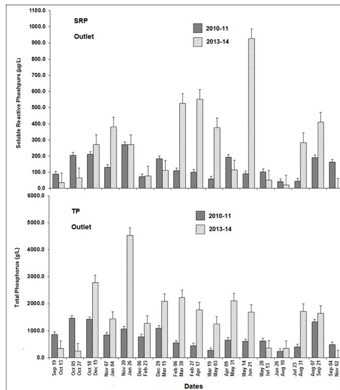
**Figure 9.** Soluble reactive phosphorus (SRP) and total phosphorus (TP) concentrations ( $\mu\text{g/L}$ ) measured at the lagoon’s outlet from 19 August 2010 to 4 September 2011 and from 13 October 2013 to 2 November 2014.
