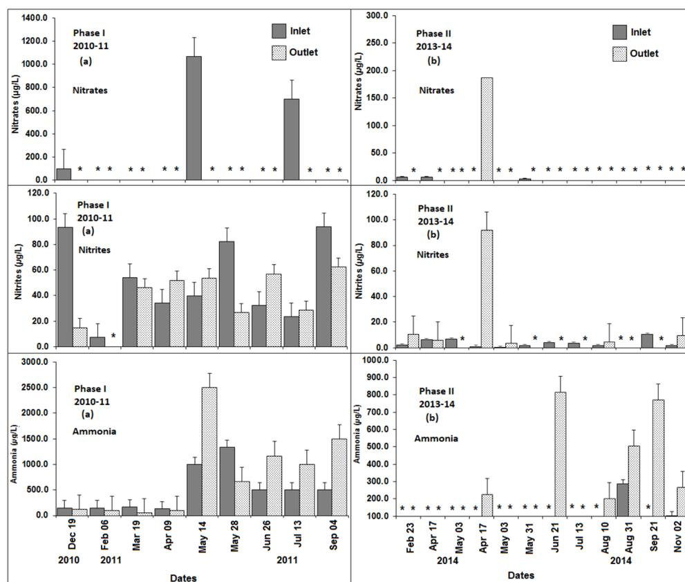
**Figure 6.** Nitrogen (nitrate, nitrite, and ammonia) from combined inlet and the lagoon’s outlet for the period of: (a) 19 December 2010 to 4 September 2011 (Phase One) and (b) 23 February 2014 to 2 November 2014 (Phase Two). (\*)Values are treated as zero (0) or if the measurable absorbance is less than the calibration range of the test.
