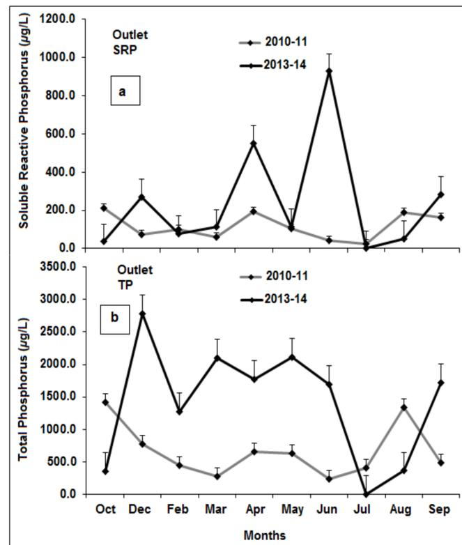
**Figure 11.** Soluble reactive phosphorus (SRP) and total phosphorus (TP) concentrations ( $\mu\text{g/L}$ ) measured at the lagoon outlet for common sampling dates during (a) 2010–2011 and (b) 2013–2014.
