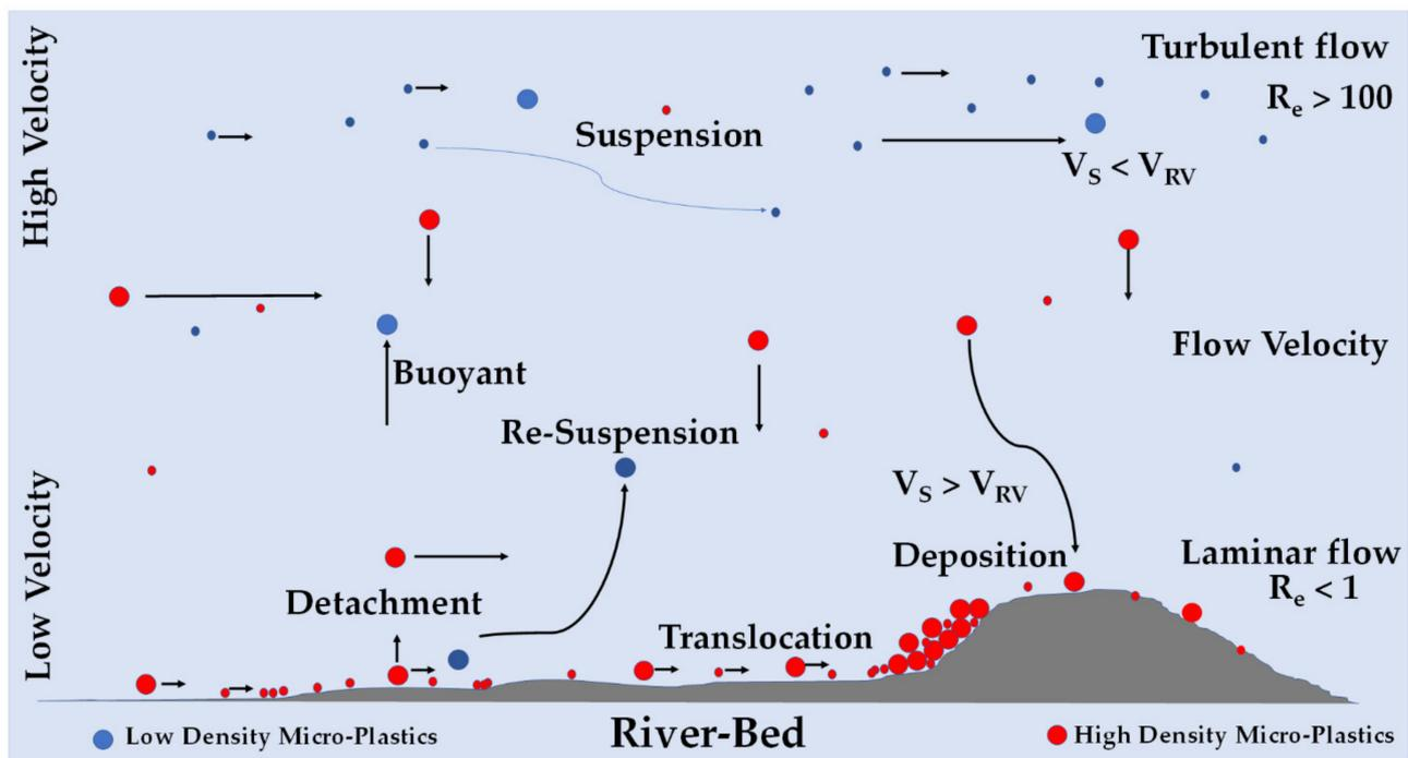
**Figure 1.** Schematic representation of natural phenomenon occurring for microplastics transport and sedimentation in rivers ( $V_S$  denotes settling velocity,  $V_{RV}$  is river velocity, and  $R_e$  is Reynolds number).
