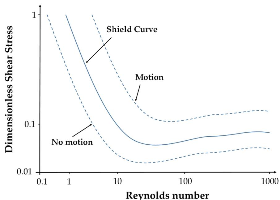
**Figure 3.** Relationship between dimensionless shear stress and Reynolds number for analyzing microplastics transport in riverine ecosystems.
