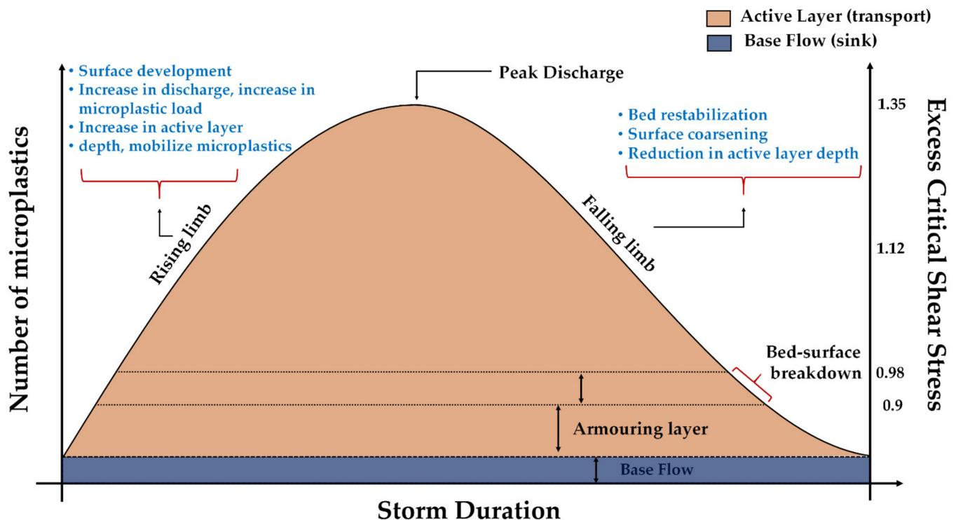
**Figure 2.** Proposing hydrograph for microplastics transport in river ecosystem and their relationship with various shear stresses of plastic particles.
