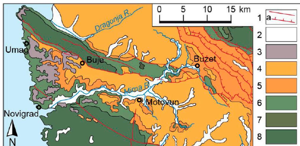
**Figure 8.** A geological map of Istria (1. Fault, 1a. Thrust, 2. Quaternary deposits (mainly Holocene), 3. Terra rossa deposits (Holocene), 4. Flysch deposits (Eocene), 5. Liburnia deposits, Foraminiferal limestone, and transitional deposits (Paleocene, Eocene), 6. Rudist limestone (Cretaceous), 7. Dolomite and breccia (Cretaceous), 8. Limestone and dolomite (Cretaceous), 9. Limestone and dolomite (Jurassic)) (taken from [31]).
