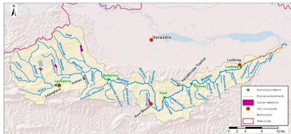
**Figure 6.** Spatial presentation of hydrological and meteorological stations in the Bednja Basin (from [21]).
