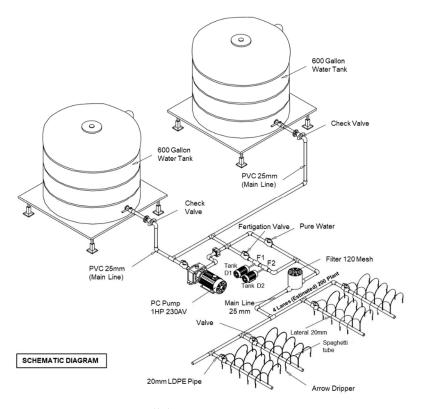
**Figure 2.** Overall drip irrigation system components.
