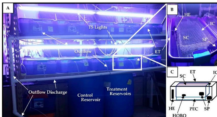
**Figure 2.** (A) Experimental tank design. (B) Treatment tank design. (C) Schematic of treatment tanks. Control Reservoir = control tank water, ET = experiment tank, HE = heating element, HOB0 = temperature and light meter, IC = incubation chamber, Outflow = IC water drainage, Outflow discharge = discharged water, PEC = plastic egg crate, SC shade cloth, SP = submersible pump, T5 lights = 54 watt lights.
