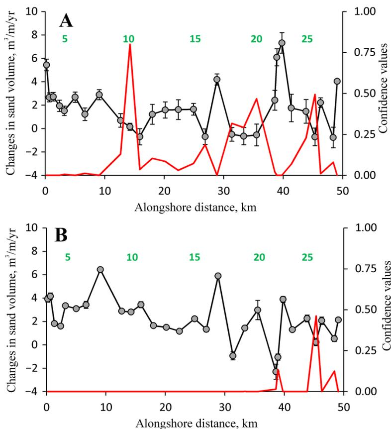
**Figure 5.** Linear trends ( $\text{m}^3/\text{m}$  per year) in the (A) beach and (B) foredune volume alongshore. Distance from Klaipėda port jetties. Red line—significance level ( $p$ -value). Green labels indicate cross-shore profile numbers.
