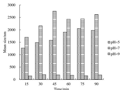
Figure 5. Mean size of nZVI with time under different pH conditions.
