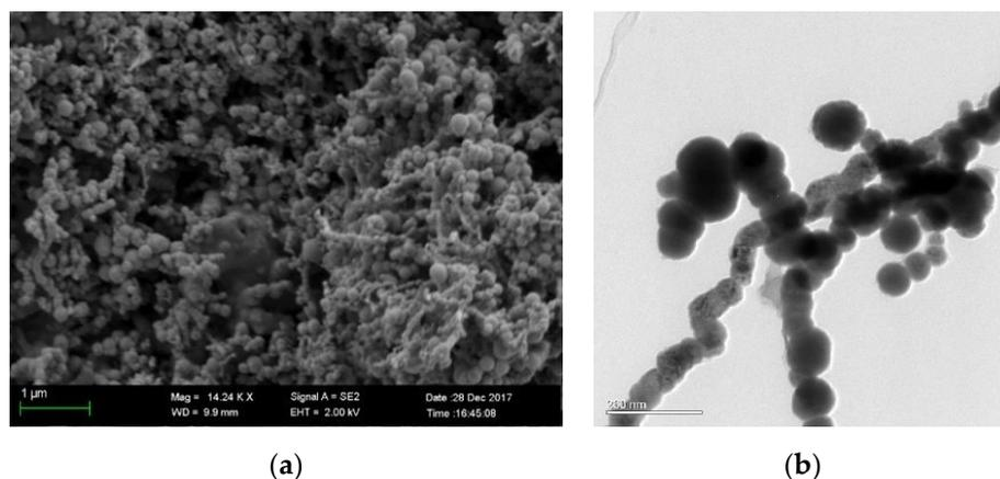
**Figure 2.** SEM and TEM images of nano zero-valent iron (nZVI) (a) SEM image (b) TEM image.
