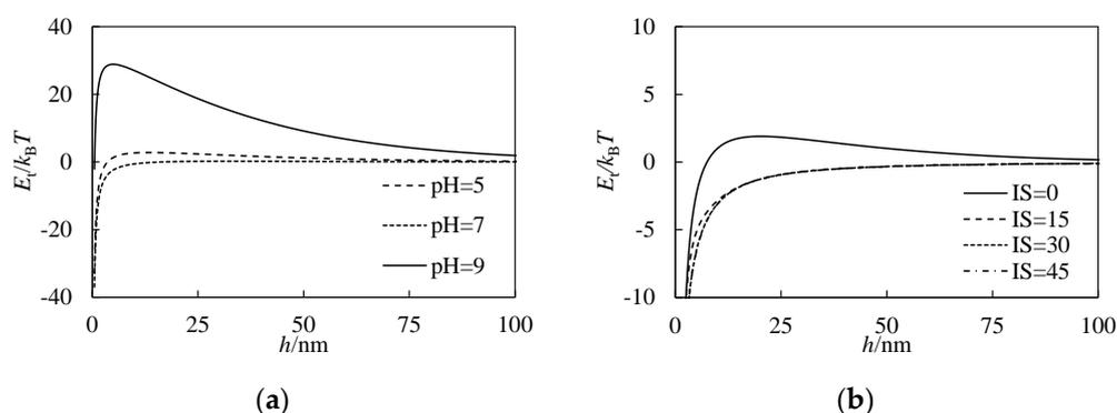
**Figure 8.** Interaction energy curves calculated by the Derjaguin–Landau–Verwey–Overbeek (DLVO) theory (a) under different pH conditions (b) under different IS conditions.
