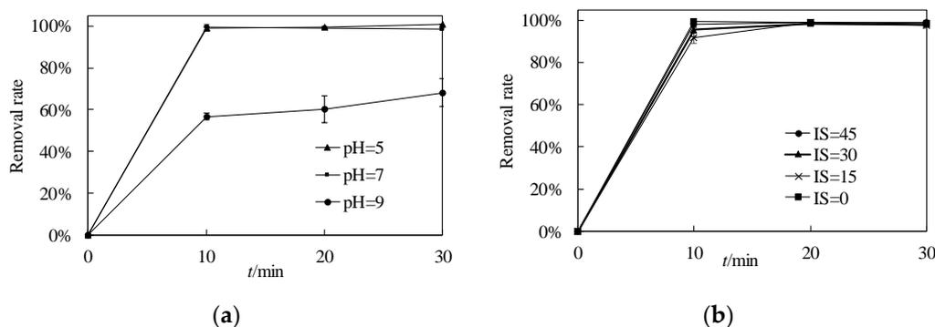
**Figure 9.** The removal rate of phosphate by nZVI with time (a) under different pH conditions (b) under different IS conditions.
