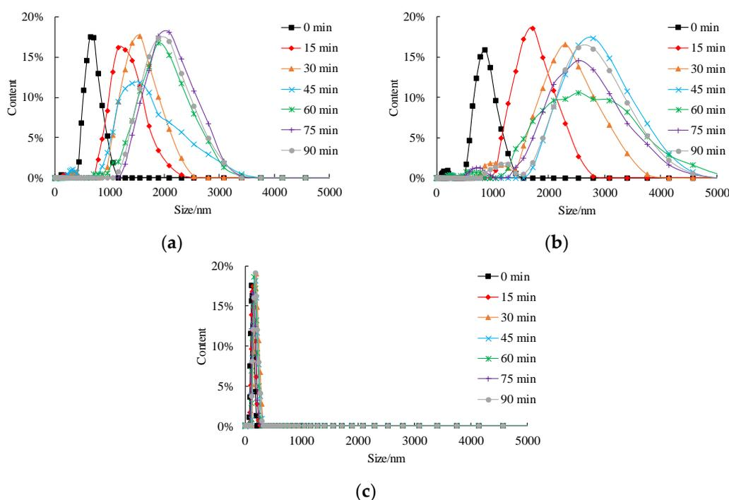
Figure 4. Influence of pH on size distribution of nZVI (a) pH = 5; (b) pH = 7; (c) pH = 9.
