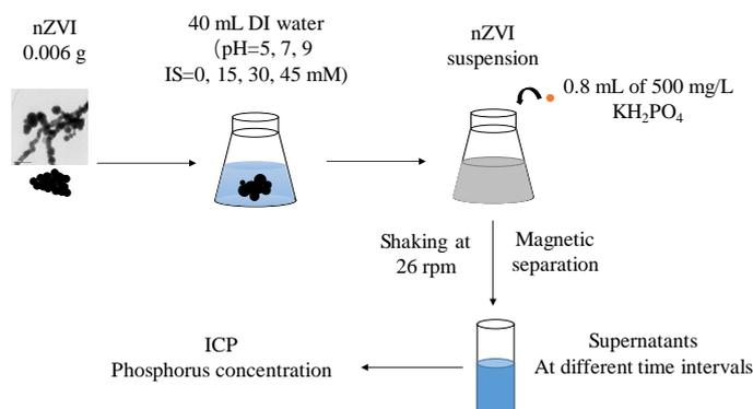
**Figure 1.** Flow chart of the batch test.
