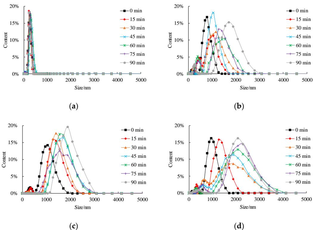
**Figure 6.** Influence of ionic strength (IS) on size distribution of nZVI (a) IS = 0 mM; (b) IS = 15 mM; (c) IS = 30 mM; (d) IS = 45 mM.
