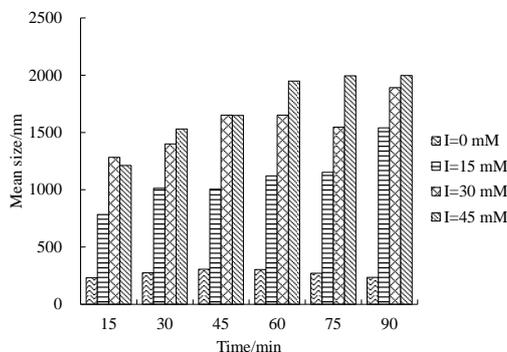
**Figure 7.** Mean size of nZVI with time under different IS conditions.
