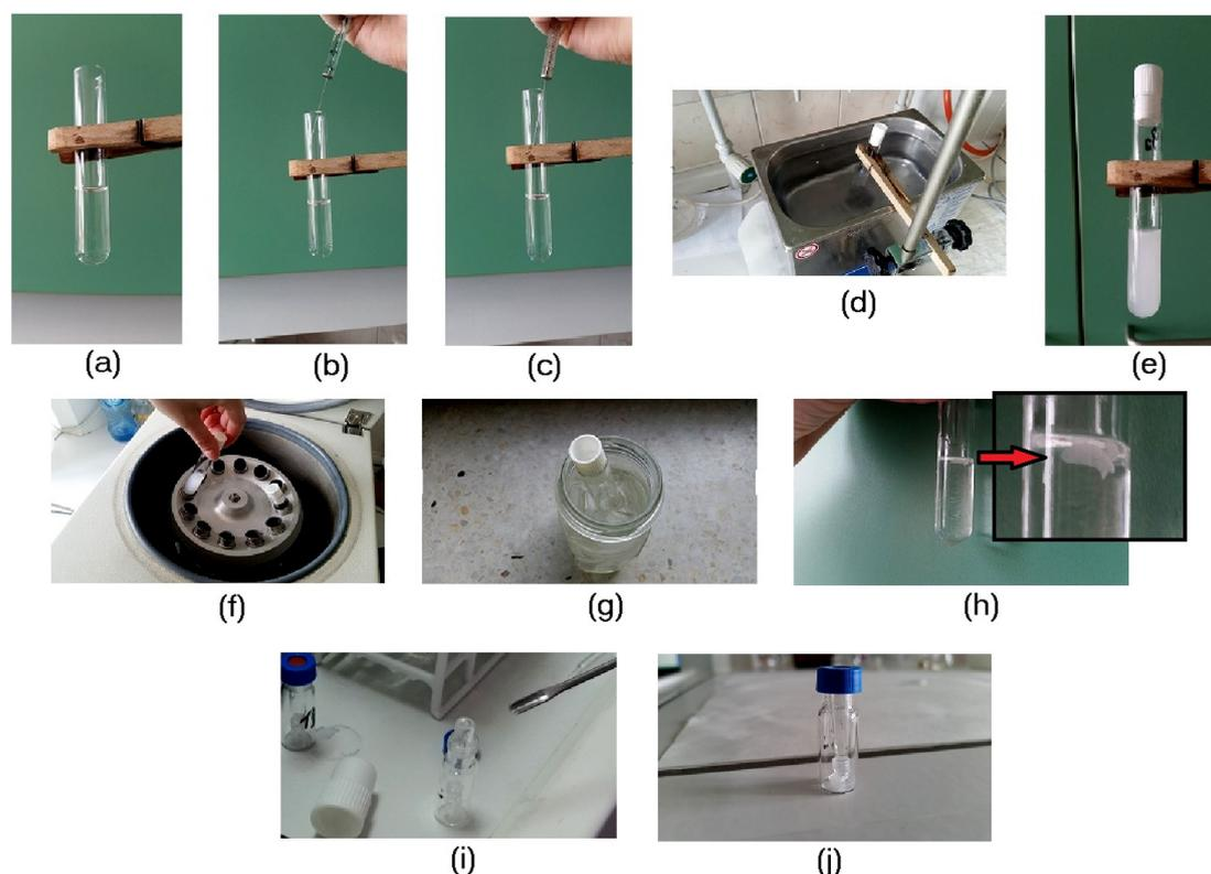
**Figure 1.** Stages of ultrasound-assisted emulsification-microextraction with solidification of the floating organic drop (USAEME-SFOD): (a) Placing test solution in a test tube; (b) adding acetic anhydride; (c) adding 1-undecanol; (d) subjecting the sample to sonication; (e) sample after sonication; (f) placing the tube in a centrifuge; (g) cooling in an ice bath; (h) a solid drop of solvent; (i) transferring the drop into a chromatography vial; (j) sample ready for GC-MS analysis.
