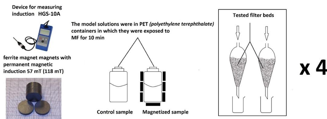
**Figure 1.** Diagram of the process of control and magnetized samples preparation.
