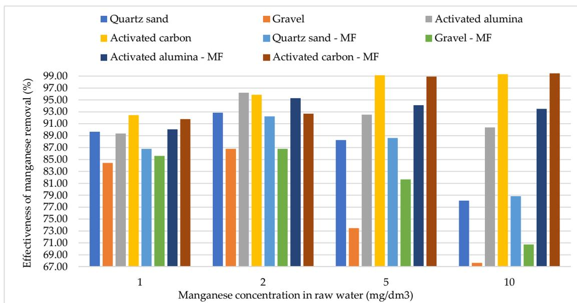
**Figure 3.** Dependence of the manganese removal efficiency on initial concentration in raw water.
