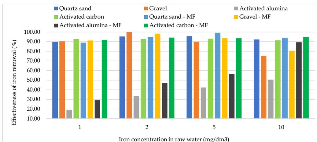
**Figure 2.** Graph of the dependence of the iron removal efficiency on initial concentration in raw water.
