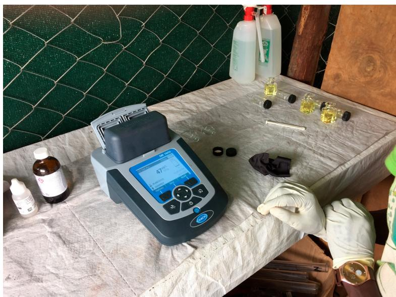
**Figure 2.** Hach *THM Plus* Method kit set up at the on-site Palorinya SWTP water quality lab (Source: Syed Imran Ali).
