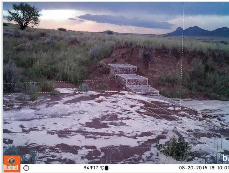
**Figure 6.** Photo taken 5 min after flow onset. Guidelines were superimposed later to assist in estimating ponding extent by C. Fandel.
