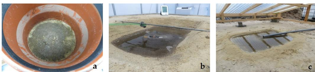
**Figure 2.** Infiltration basin: column (a), laboratory tank (b) and field infiltration unit (c).
