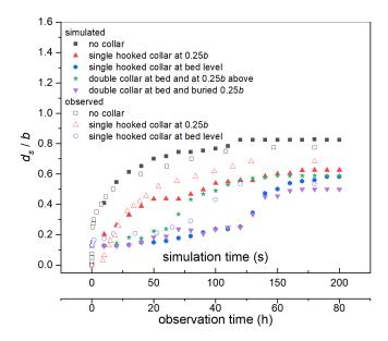
Figure 4. Scour development for the different hooked-collar configurations.
