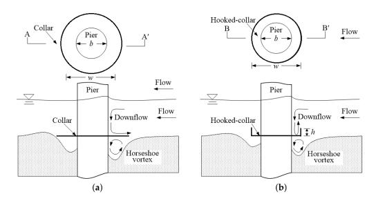
Figure 1. Flow features around piers: (a) pier fitted with a collar; and (b) pier fitted with a hooked-collar.
