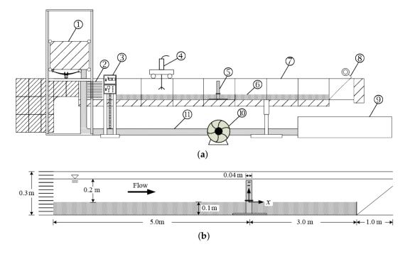
**Figure 2.** The flume system used for the experiments: (**a**) side view and (**b**) schematic diagram of the bridge pier and coordinate system. 1. Head tank. 2. Flow straightener. 3. Control panel. 4. Acoustic Doppler Velocimeter (ADV). 5. Pier. 6. Sediment bed. 7. Main channel. 8. Tailwater gate. 9. Re-circulating tank. 10. Pump. 11. Re-circulating pipe.
