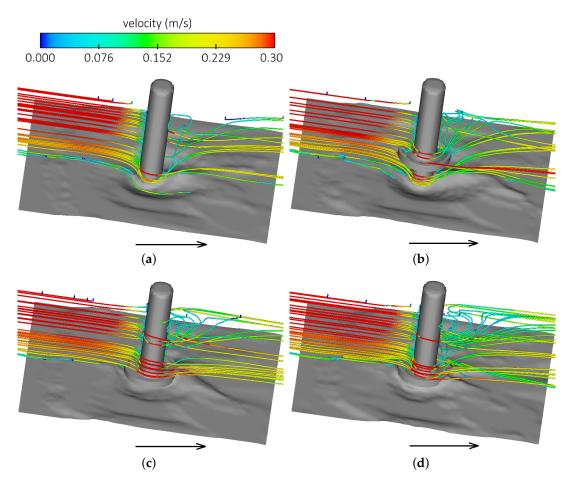
**Figure 7.** Visualization of streamlines: (**a**) no hooked-collar; (**b**) single hooked-collar at 0.25b; (**c**) single hooked-collar at bed level; and (**d**) double collar at the bed and buried -0.25b.
