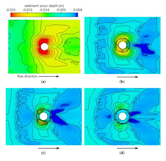
**Figure 8.** Contours of scour depth: (a) no hooked-collar; (b) single hooked-collar at 0.25b; (c) single hooked-collar at bed level; and (d) double collar at the bed and buried -0.25b.
