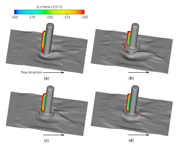
**Figure 6.** Visualization of vortices: (**a**) no hooked-collar; (**b**) single hooked-collar at 0.25*b*; (**c**) single hooked-collar at bed level; and (**d**) double collar at the bed and buried 0.25*b*.
