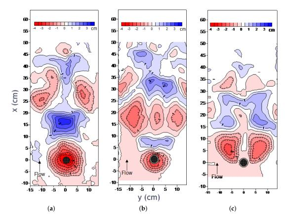
**Figure 5.** Observed scour pattern around the piers: (**a**) bridge pier without the hooked-collar; (**b**) pier with the hooked-collar positioned 0.25*b* above bed; and (**c**) pier with the hooked-collar positioned at bed level.
