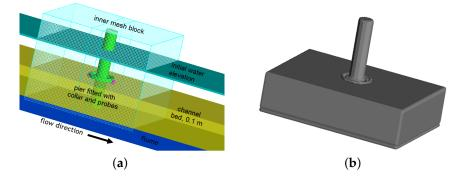
**Figure 3.** An example of (**a**) a bridge pier and the hooked-collar installation, as well as the inner mesh block and (**b**) favorized image showing the hooked-collar geometry.
