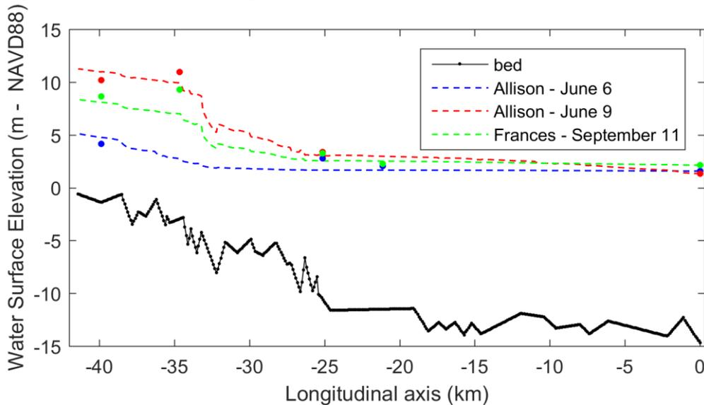
**Figure S5.** Comparison of the maximum water levels observed for Tropical Storm Allison and Frances with the results from the 1-D hydraulic model.
