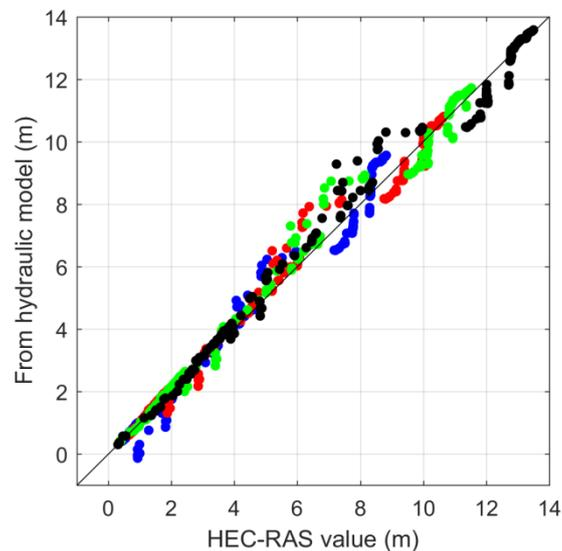
**Figure S3.** Scatter plot of the water levels obtained from the simplified hydraulic model developed in this study versus the results from HEC-RAS for the 10-year (blue), 50-year (red), 100-year (green), 500-year (black) return period as derived by FEMA and HCFCD.
