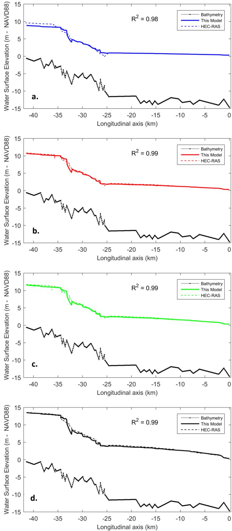
**Figure S4.** Comparison of the simplified hydraulic model developed in this study with the results from HEC-RAS for riverine boundary conditions for the 10-year (a), 50-year (b), 100-year (c), 500-year (d) return period as derived by FEMA and HCFC.
