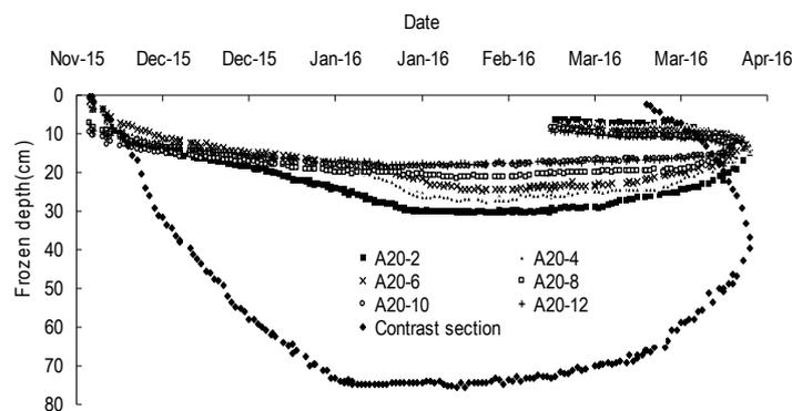
Figure 6. Change process lines of the frozen depths under the different EPS thicknesses.
