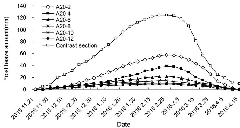
**Figure 2.** Change process lines of the frost heave amounts using different EPS treatments.
