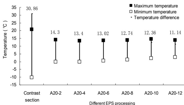
**Figure 5.** Temperature extremum and temperature difference values of the EPS with different thicknesses.
