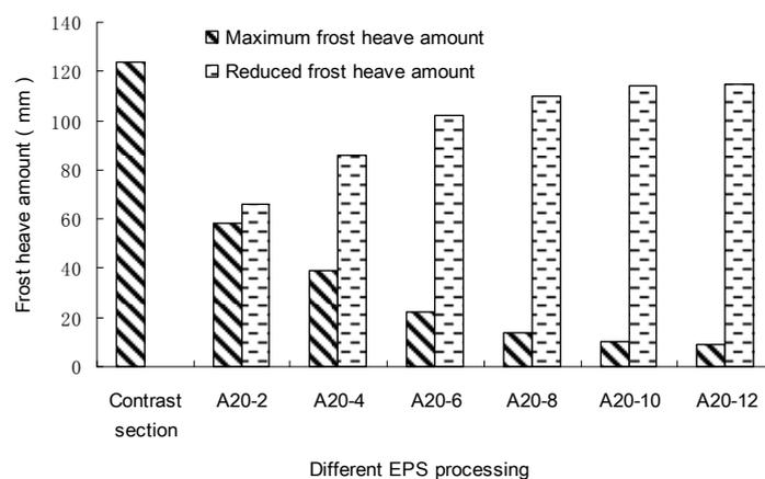
**Figure 3.** Maximum frost heave amount and reduced frost heave amounts with the different EPS processing procedures.
