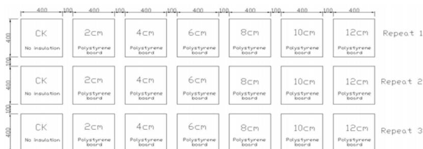
**Figure 1.** Planar layout of different treatment blocks.
