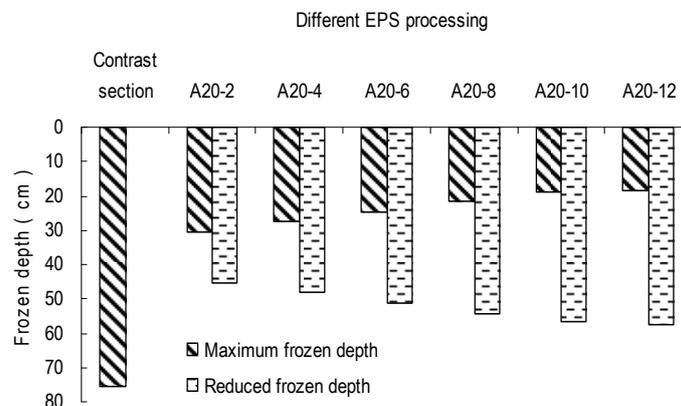
Figure 7. Maximum frozen depth and reduced frozen depths under the different EPS thicknesses.
