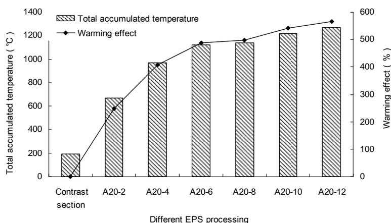
**Figure 4.** Total accumulated temperature and warming effects of the EPS with different thicknesses.
