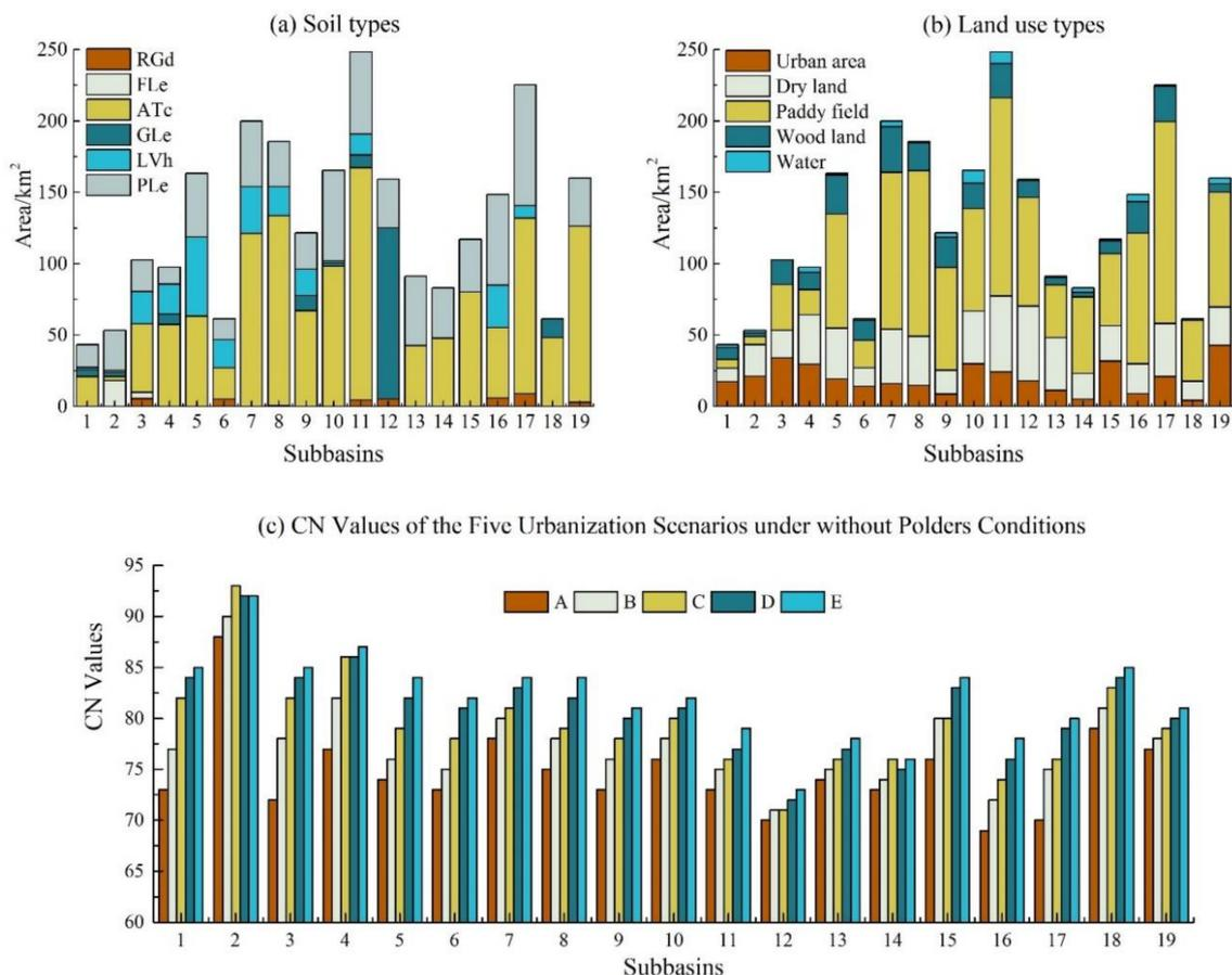
**Figure 4.** The areas of soil types and land uses in the sub basins of the Qinhuai River basin (scenario B) and the CN values of the five urbanization scenarios under without polder conditions (a) soil types (scenario B), (b) land use types (scenario B), (c) CN values under without polder conditions.
