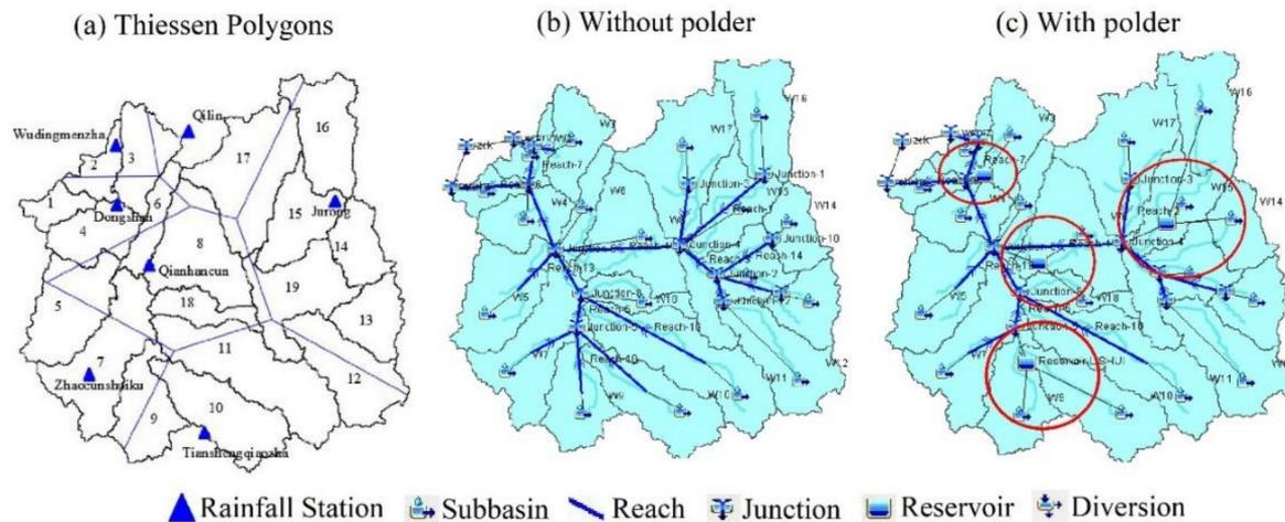
**Figure 2.** Thiessen polygons of the Qinhuai River basin and HEC-HMS models of the Qinhuai River basin under both with and without polder conditions, (a) Thiessen polygons of the Qinhuai River basin, (b) HEC-HMS model under without polder condition, (c) HEC-HMS model under with polder condition.
