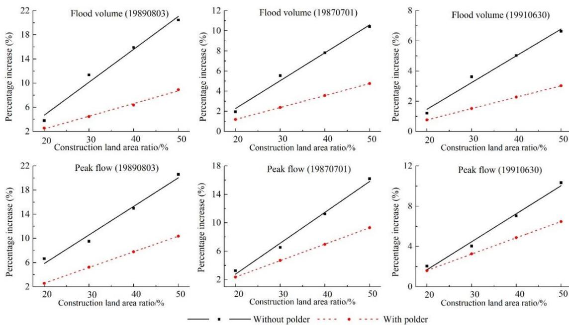
**Figure 5.** The potential changes of percentage increases in  $Q_v$  and  $Q_p$  from scenario A under the without polder and with polder conditions for different flood magnitudes.
