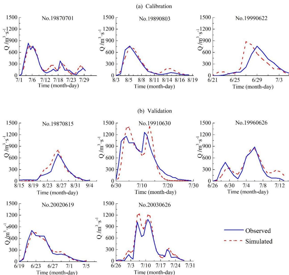
**Figure 3.** Comparison of simulated and observed hydrographs for the selected eight flood events (a) calibration period, (b) validation period.
