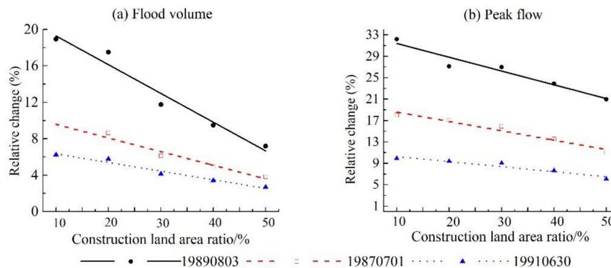
**Figure 6.** The potential changes of relative change in  $Q_v$  and  $Q_p$  between with and without polder conditions for different flood magnitudes under different urbanization scenarios (a) flood volume, (b) peak flow.
